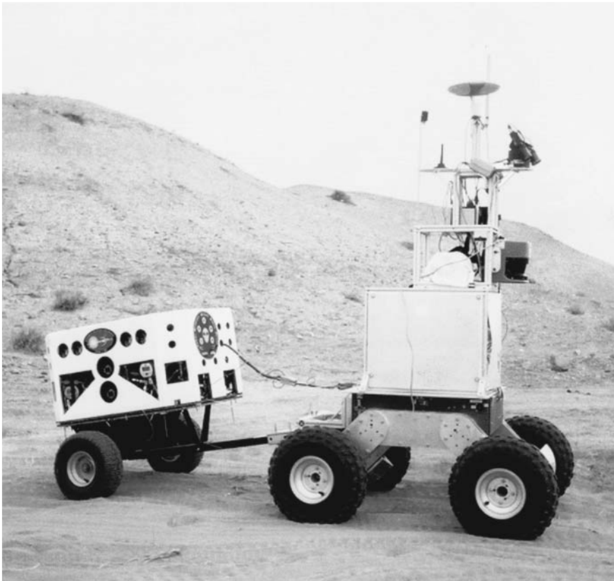
fuel cell Deriving electricity from reverse electrolysis, the fuel cell has proven to be a valuable source of power, with potential applications in space travel and for automotive transportation. This model is used to power an experimental “robotic assistant” for future manned missions to the Moon or Mars. National Aeronautics and Space Administration
