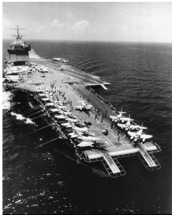
aircraft carrier First developed at the end of World War I, aircraft carriers evolved over the next decades into the largest warships afloat. Here the nuclear powered U.S.S. Enterprise launches A-4 Skyhawk bombers. National Archives and Records Administration
