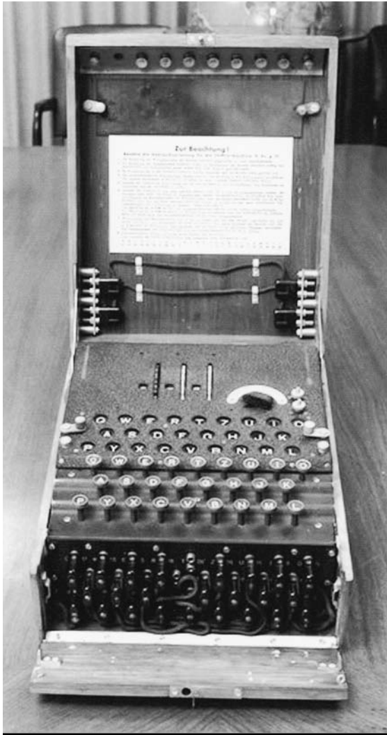
encryption machine The German Enigma machine was supposed to produce unbreakable codes, but its system of transposing letters was cracked, first by the Poles in the 1930s and then by the British, using early analog computers at Bletchley Park. National Security Agency
