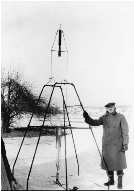
liquid-fueled rocket Robert Goddard, an American scientist who calculated the force required to escape Earth’s gravity, prepares to fire his first liquid-fueled rocket in 1926. National Aeronautics and Space Administration
