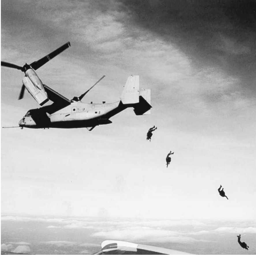
vertical takeoff and landing aircraft The tilt-rotor Osprey V-22 can take off vertically and, by turning the wing and rotor assembly, fly forward as a conventional aircraft. In this practice run, troops parachute from the ascending aircraft. U.S. Navy
