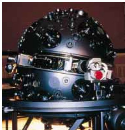
CUSTOMIZED ZEISS PROJECTOR at the planetarium can duplicate scintillation—the twinkling of stars.
