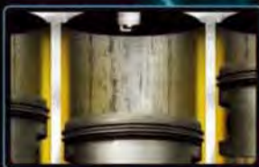
Wear Cuts Scratches in Cylinders Causing Compression Loss
