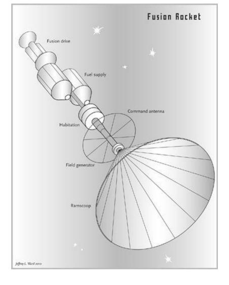
A ramjet fusion engine, because it scoops hydrogen from interstellar space, can theoretically run forever. (photo credit 6.2)
