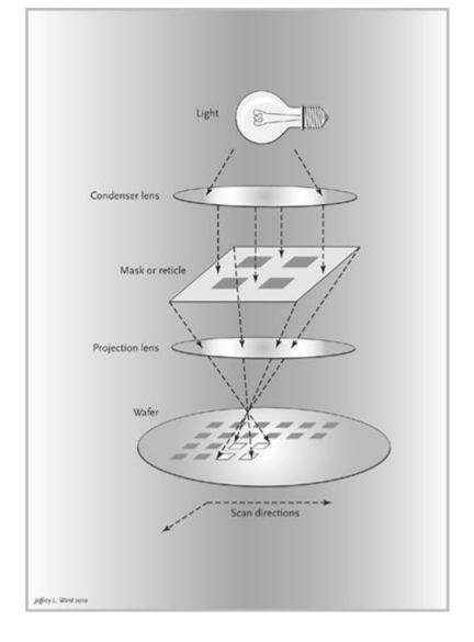
The end of Moore's law. Chips are made the same way as designs on T-shirts. Instead of spray painting over a stencil, UV light is focused on a stencil, burning an image onto layers of silicon. Acids then carve out the image, creating hundreds of millions of transistors. But there is a limit to the process when we hit the atomic scale. Will Silicon Valley become a rust belt? (photo credit 1.1)
