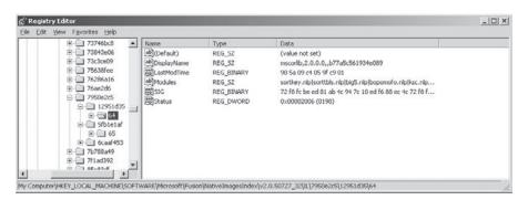
FIGURE 8.19 Binding to the Native Image of mscorlib.dll (the Registry IL Section)
