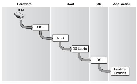
FIGURE 9.4 Chain of Trust Using a TPM
