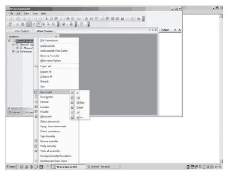
FIGURE 3.5 Using Spices.NET to Decompile an Executable to a Specific Language
