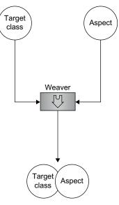
FIGURE 4.4 Using AOP Weaving to Inject External Aspect Code into a Class
