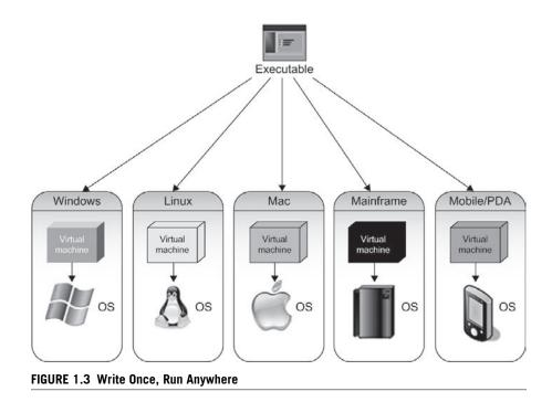
Figure 1.3 illustrates the same application running on the Windows, Linux, Mac, mainframe, and mobile/PDA platforms, while letting the VM tied to those specific platforms bridge the application and the OS.
