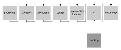
FIGURE 4.3 Hooking into the JIT Compiler to Influence the Generated Native Machine Code
