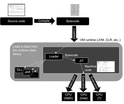
FIGURE 1.2 Typical Execution Model of a Managed VM Runtime
