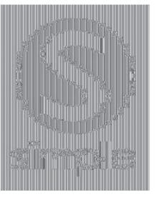
FIGURE 5.11 Encrypted Image (Using ECB Mode)
