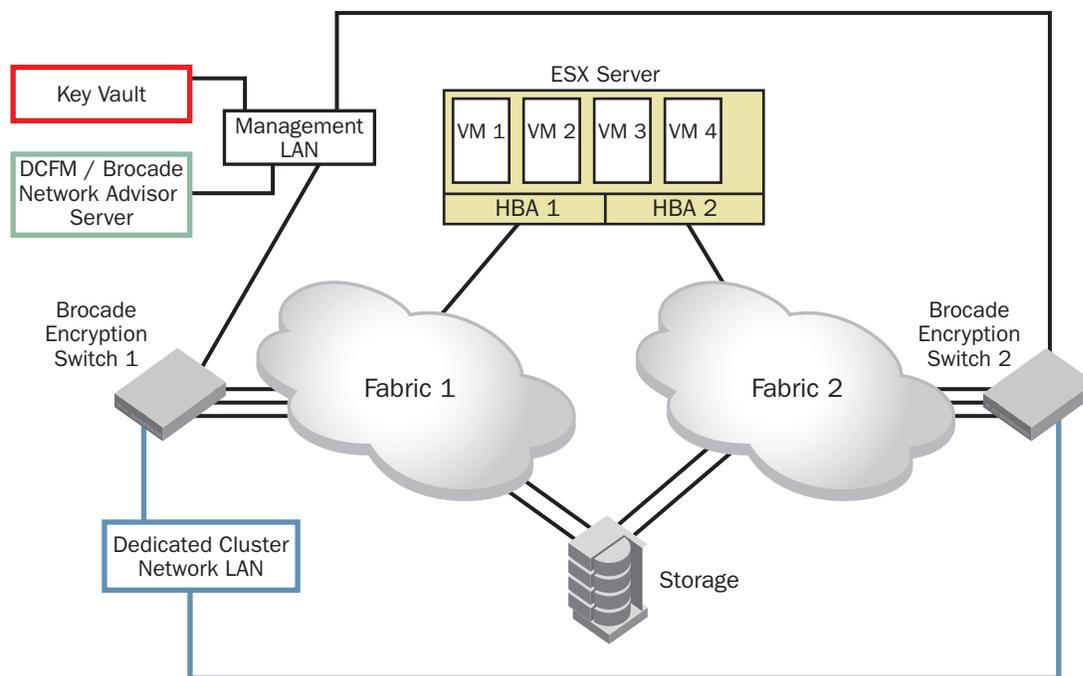
Figure 18. Dual-path connection between ESX server and storage.
