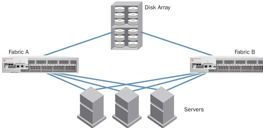
Figure 20. Dual-fabric SAN with only one Brocade Encryption Switch making up each fabric.
