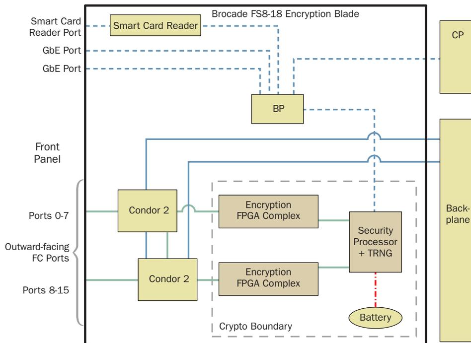
Figure 15. Brocade FS8-18 Encryption Blade internal architecture.
