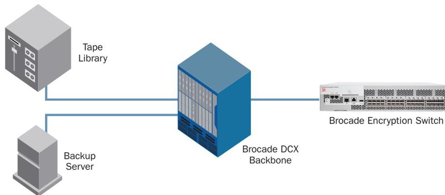
**Figure 22.** Tape backup SAN with a Brocade Encryption Switch.
