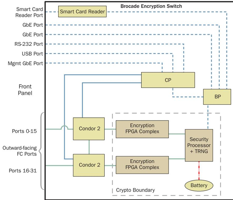
Figure 14. Brocade Encryption Switch internal architecture.
