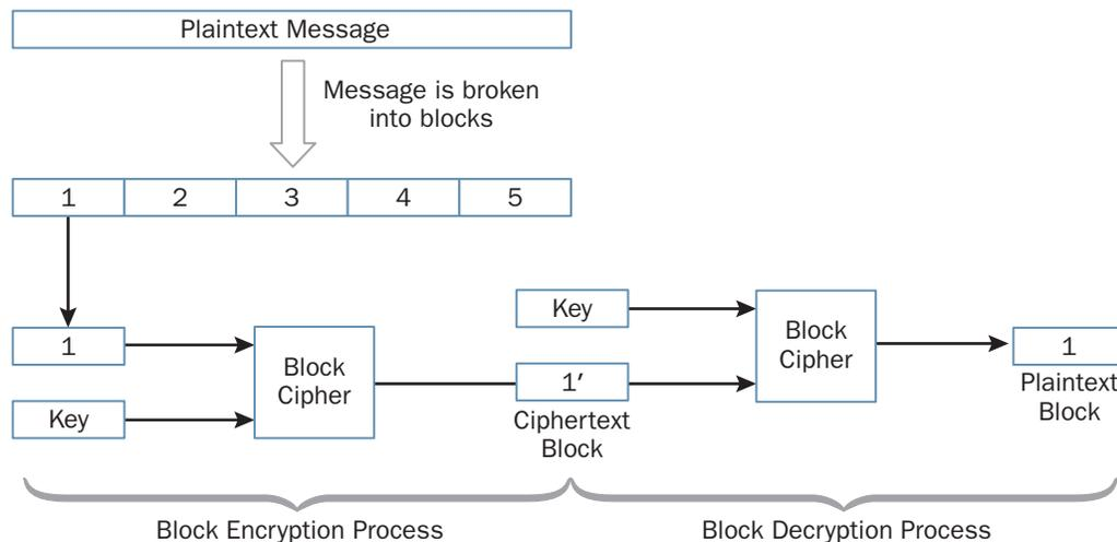
Figure 4. Block cipher encryption/decryption.
