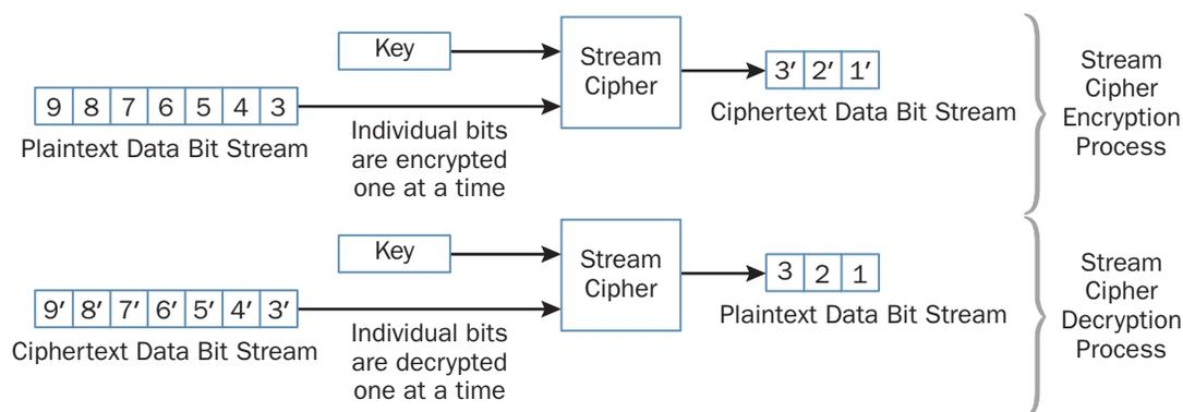
Figure 5. Stream cipher encryption/decryption.
