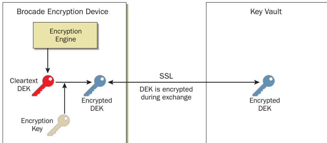
**Figure 3.** Opaque key exchange.
