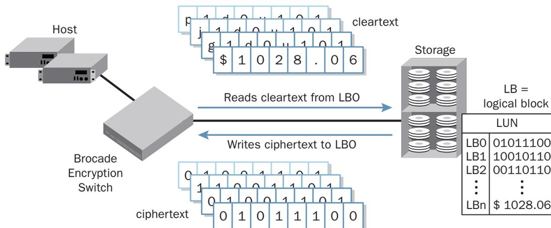
**Figure 11.** First-time encryption operation illustrating the FTE process.
