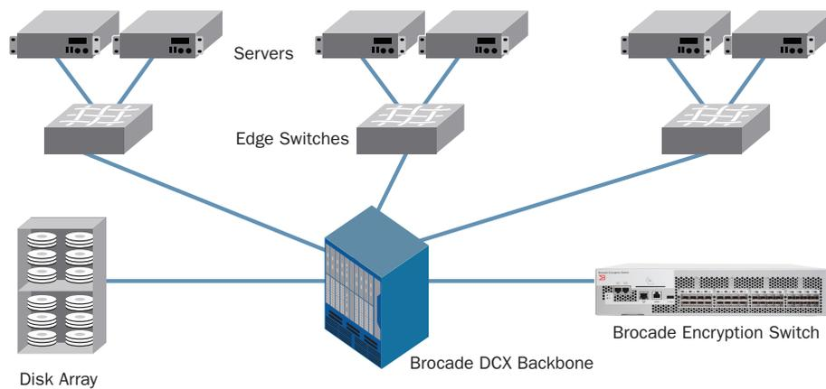
**Figure 21.** Integrating a Brocade Encryption Switch into an existing fabric.
