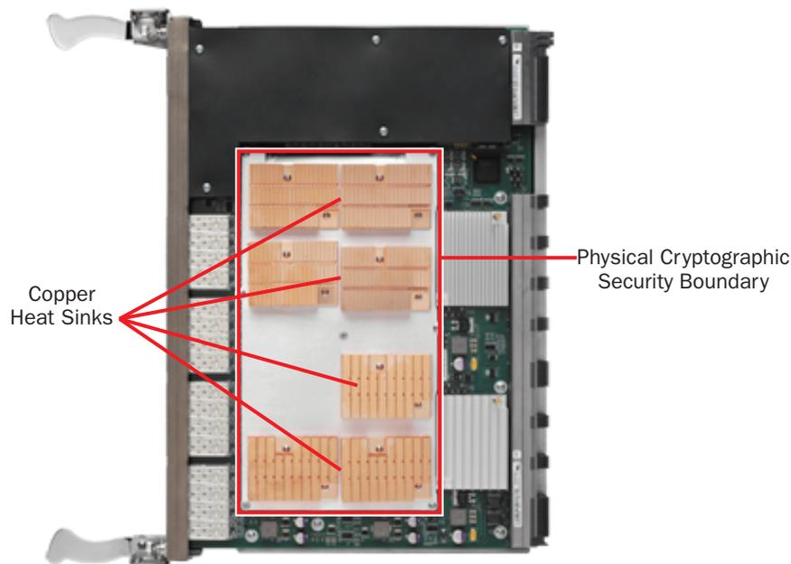
**Figure 10.** Side view of the Brocade FS8-18 Encryption Blade.
