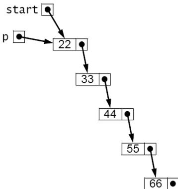
Figure 3.14 Initializing `p` at the `start` node
