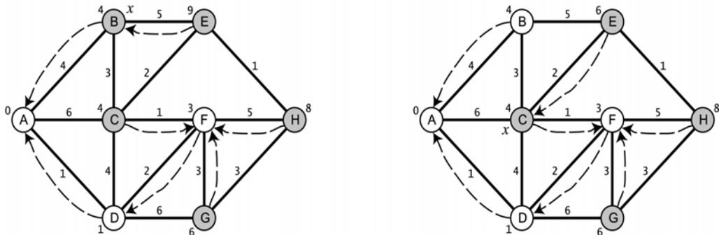
Figure 15.26 The fourth and fifth iterations of Dijkstra's algorithm
