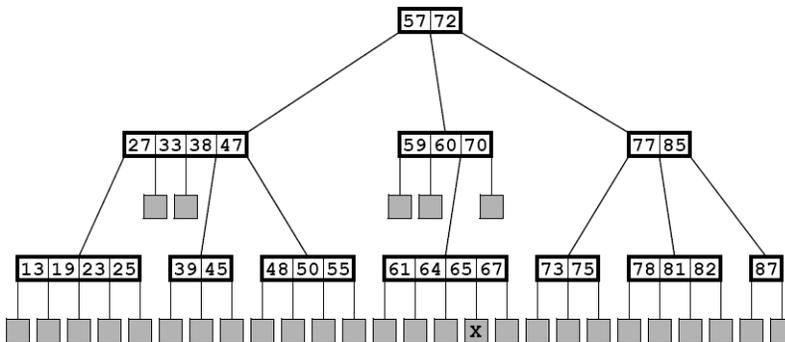
Figure 12.2 Inserting 66 into a five-way search tree
