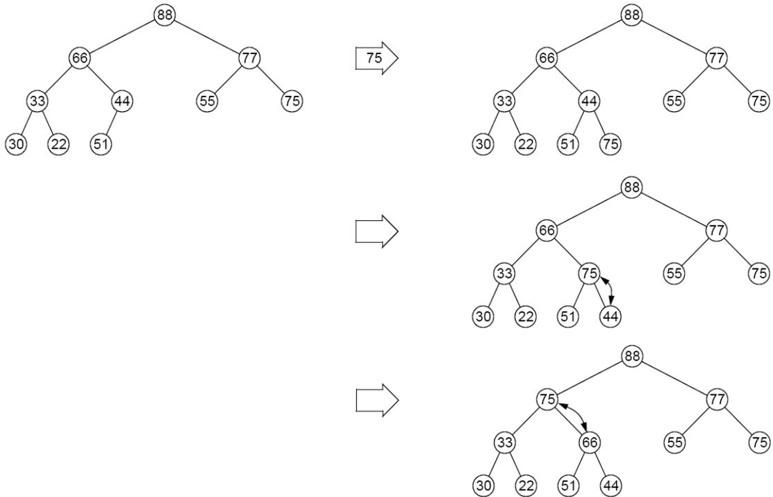
Figure 13.5 Inserting 75 into a heap
