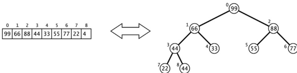
Figure 14.3 The natural mapping for the heap sort
