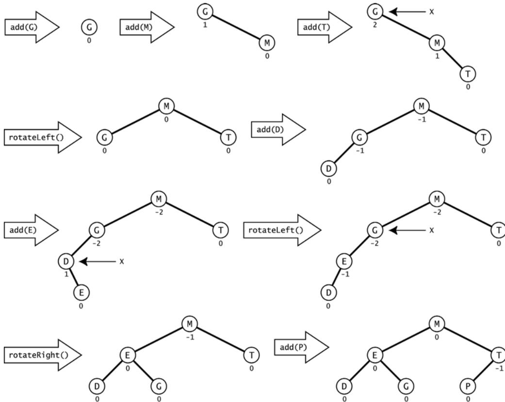
**Figure 12.13 Inserting into an AVL tree**
