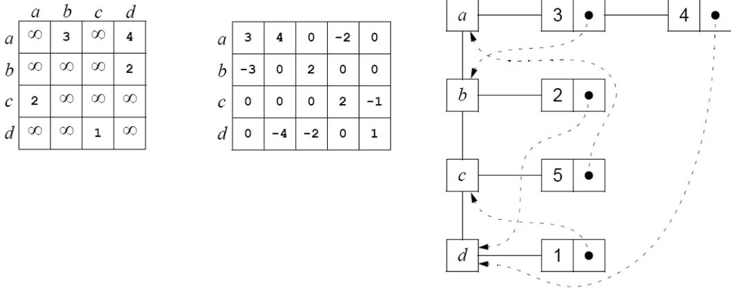
Figure 15.21 Adjacency matrix, incidence matrix, and adjacency list
