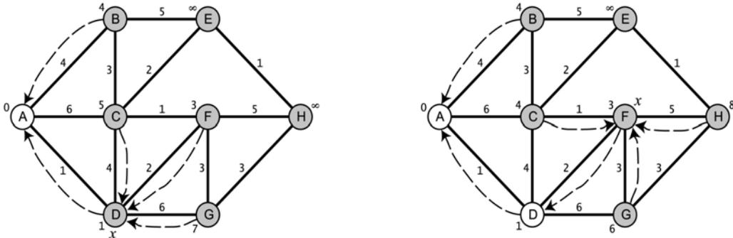
Figure 15.25 The second and third iterations of Dijkstra's algorithm
