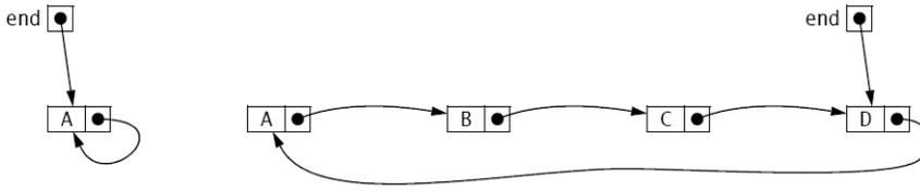
Figure 7.2 The end reference in the Ring class
