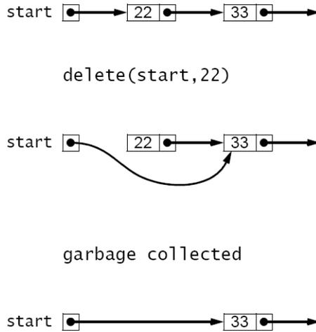
Figure 3.23 Deleting the first element from a sorted linked list
