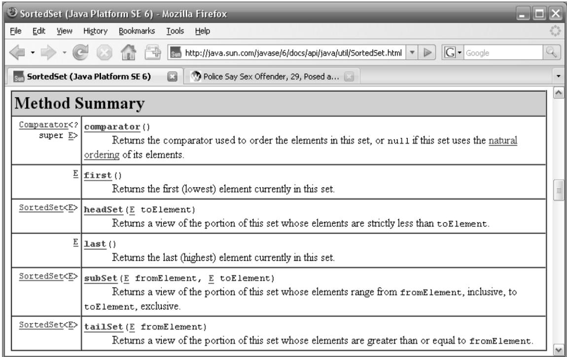
Figure 4.6 Specialized methods specified by the `java.util.SortedSet` interface
