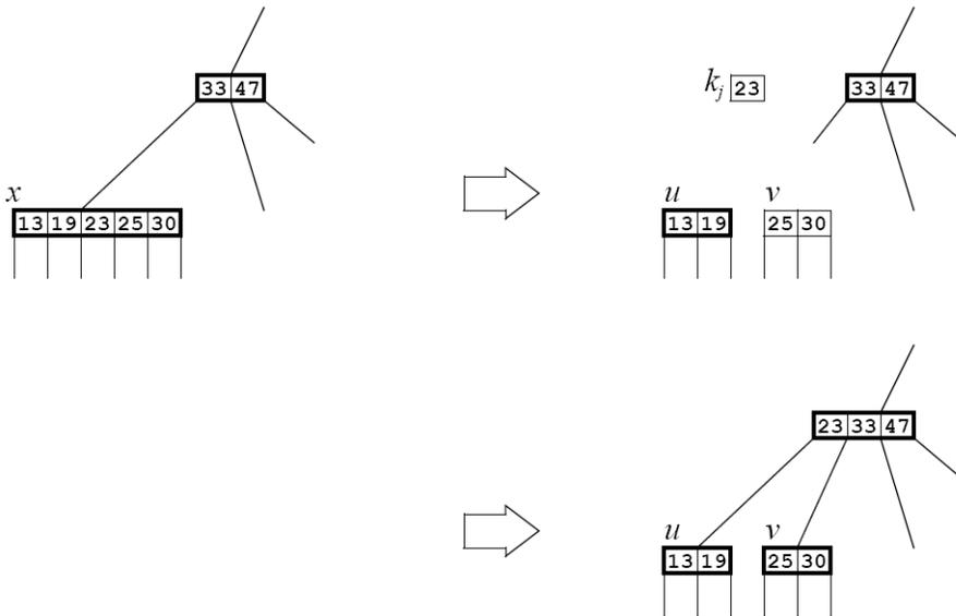
Figure 12.6 Inserting into a B-tree
