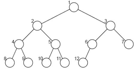
Figure 13.3 Array indexes in a heap
