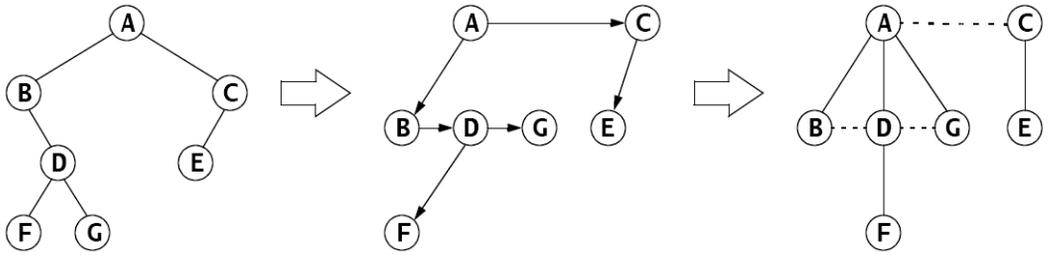
Figure 11.40 Mapping a forest into a binary tree
