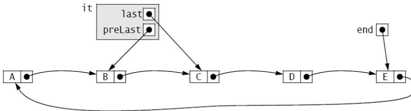
Figure 7.3 The last and preLast references in the RingIterator class
