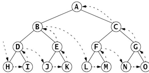
Figure 11.17 The postorder traversal of a binary tree
