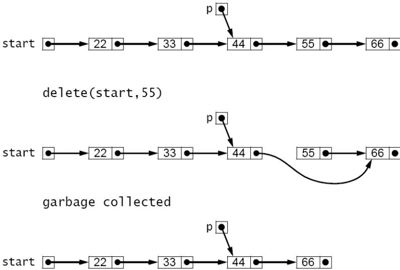
Figure 3.24 Deleting any other element from a sorted linked list
