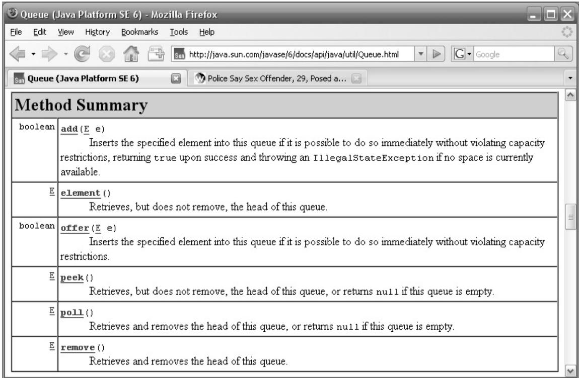
Figure 4.10 Specialized methods specified by the `java.util.Queue` interface
