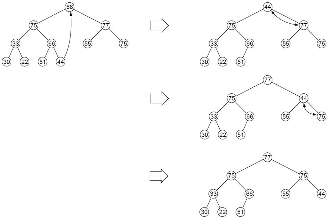
Figure 13.6 Deleting 88 from a heap
