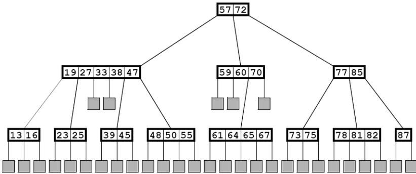
Figure 12.17 Inserting the key 16 in a five-way search tree
