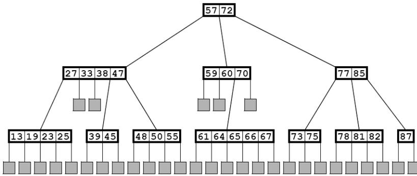
Figure 12.3 Inserting 66 into a five-way search tree
