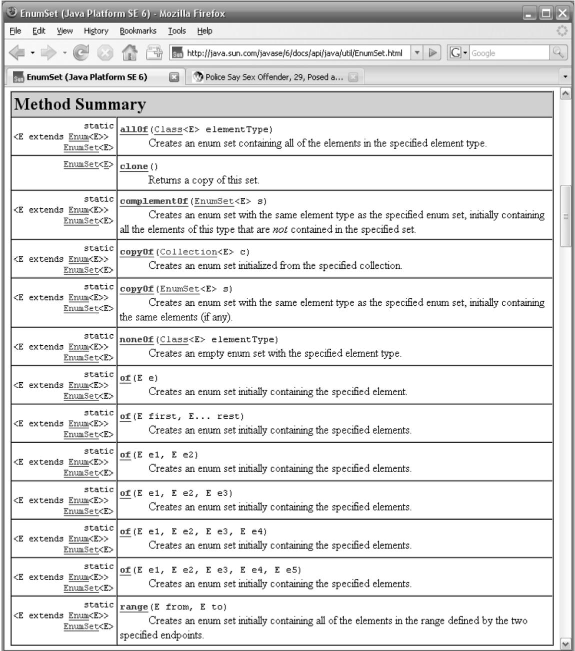
Figure 4.8 Specialized methods implemented by the java.util.EnumSet class
