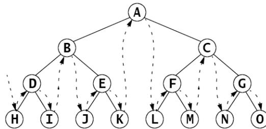
Figure 11.18 The inorder traversal of a binary tree
