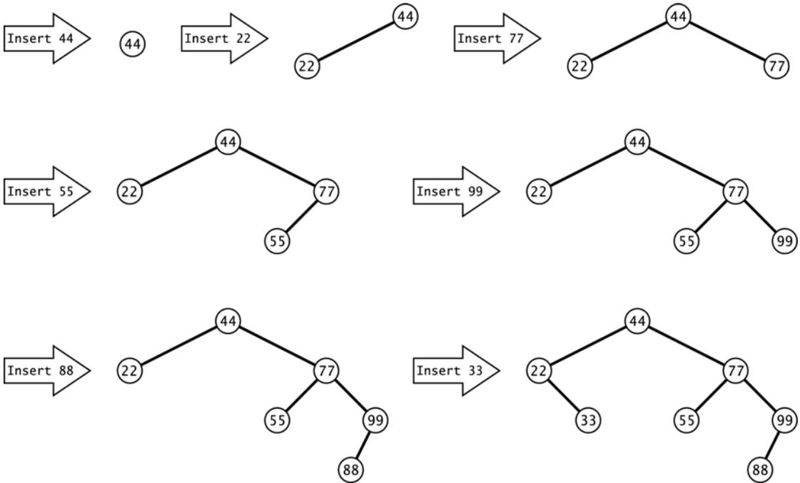
Figure 12.9 Inserting into a binary search tree
