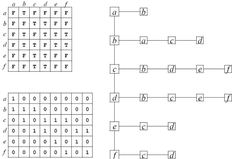
Figure 15.47 Adjacency matrix, incidence matrix, and adjacency list
