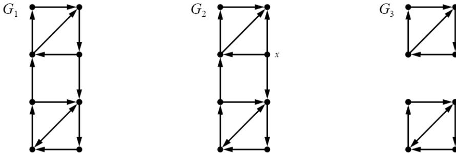
Figure 15.19 Strongly connected and weakly connected components
