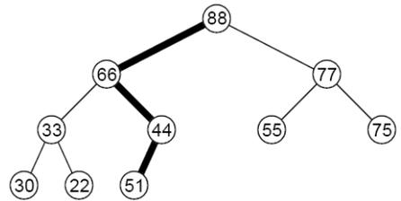
Figure 13.4 Checking the heap property
