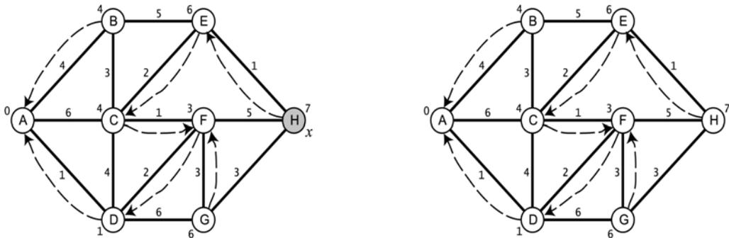
Figure 15.28 The last two iterations of Dijkstra's algorithm
