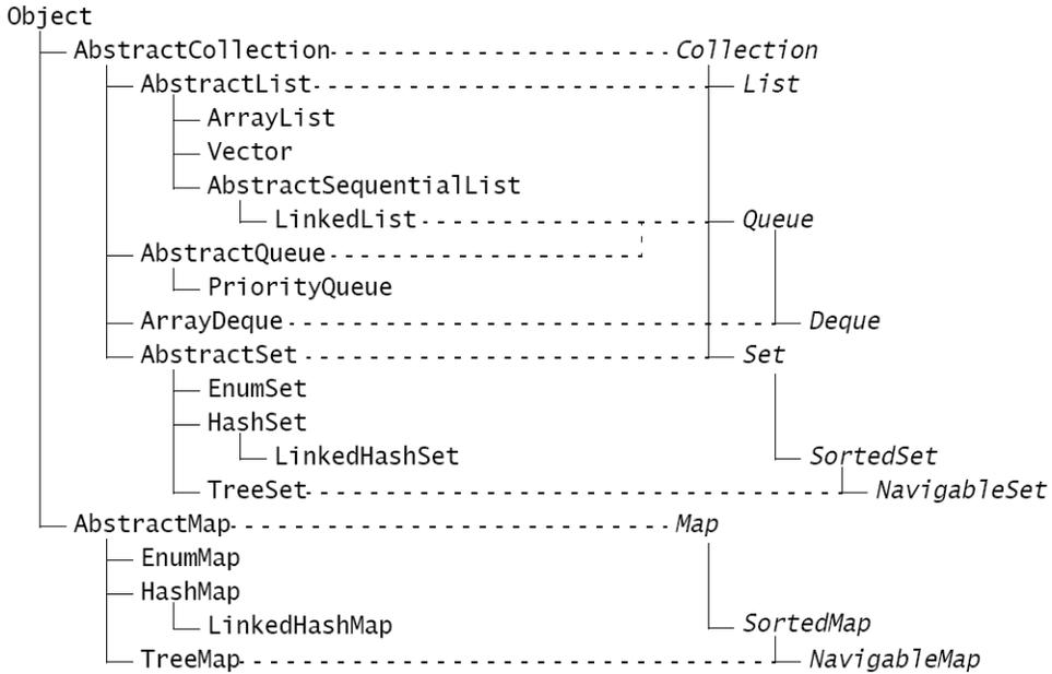
Figure 4.1 The inheritance hierarchy for the Java Collections Framework
