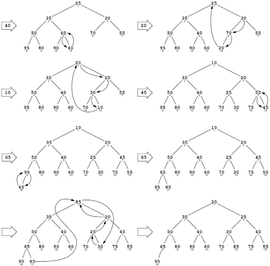
Figure 13.12 (continued) Insertion into a heap
