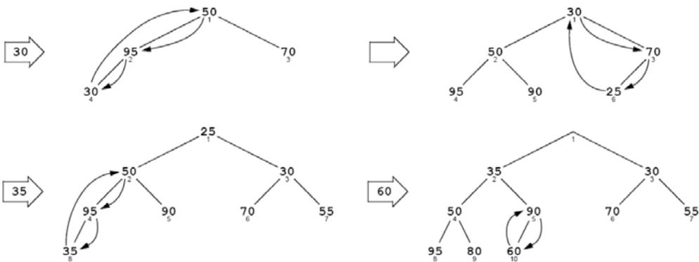
Figure 13.12 Insertion into a heap
