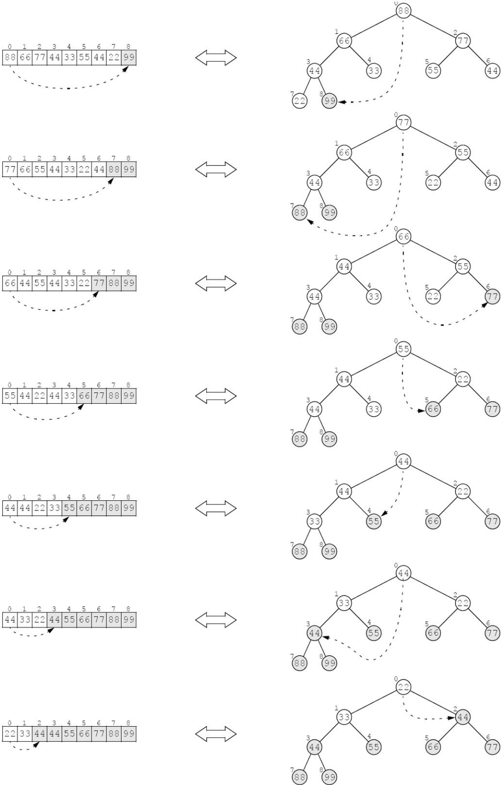
Figure 14.4 Tracing the heap sort
