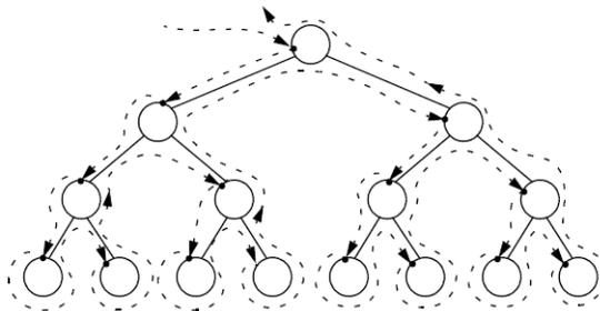
Figure 11.16 The preorder traversal of a binary tree
