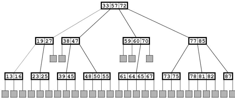
Figure 12.18 Inserting the key 16 in a five-way search tree
