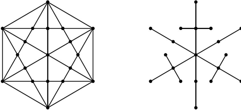
Figure 15.6 The graph on the right is a spanning tree of the graph on the left
