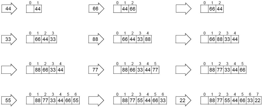
Figure 13.10 Trace of heap insertions into an array
