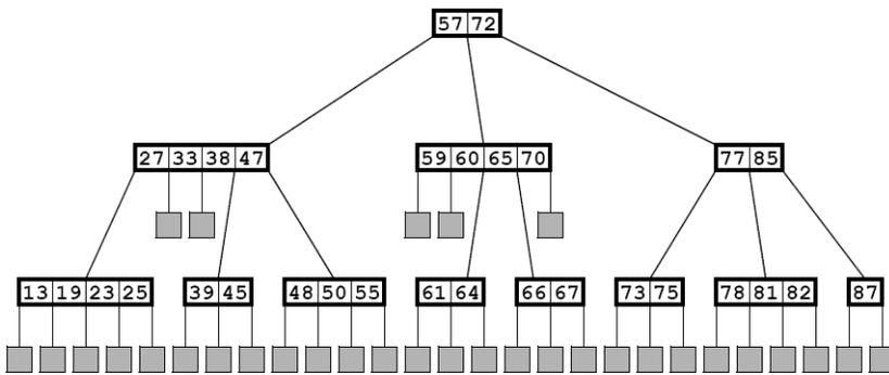
Figure 12.4 Inserting 66 into a five-way search tree
