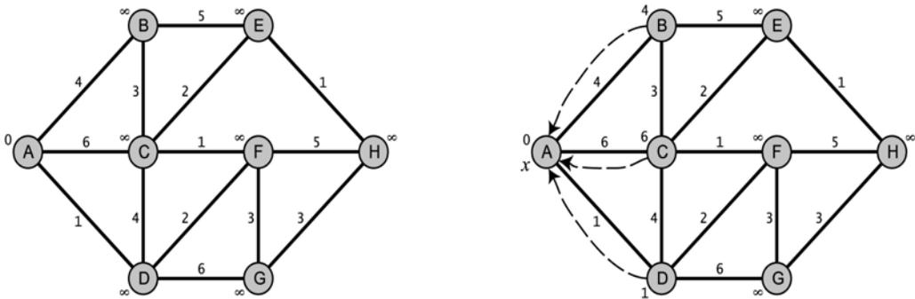
Figure 15.24 The first iteration of Dijkstra's algorithm
