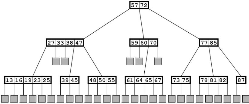
Figure 12.16 Inserting the key 16 in a five-way search tree
