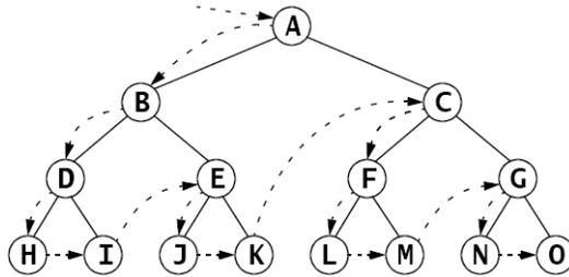
Figure 11.15 The preorder traversal of a binary tree
