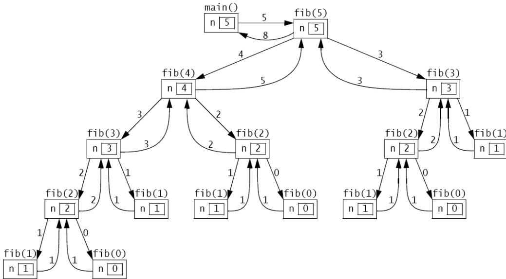
Figure 9.2 Tracing the recursive Fibonacci function
