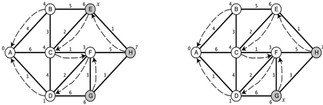
Figure 15.27 The sixth and seventh iterations of Dijkstra's algorithm
