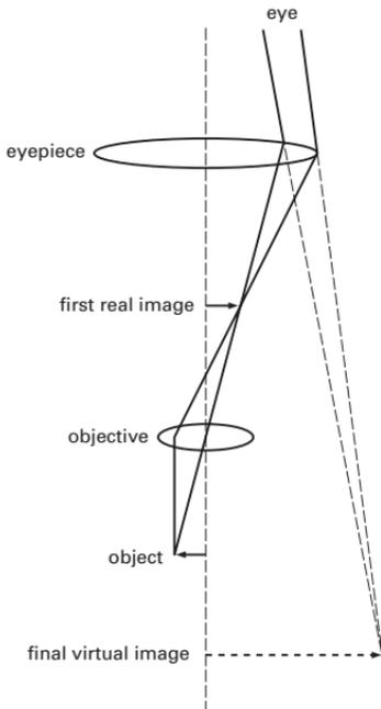
**Microscope.** Compound microscope.
