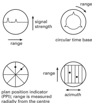
**Radar.** Types of cathode-ray tube radar display.
