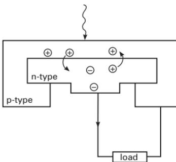
**Solar cell.** A silicon *p-n* junction.
