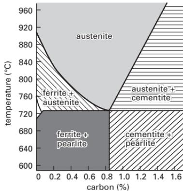
**Steel.** Phase diagram for steel.
