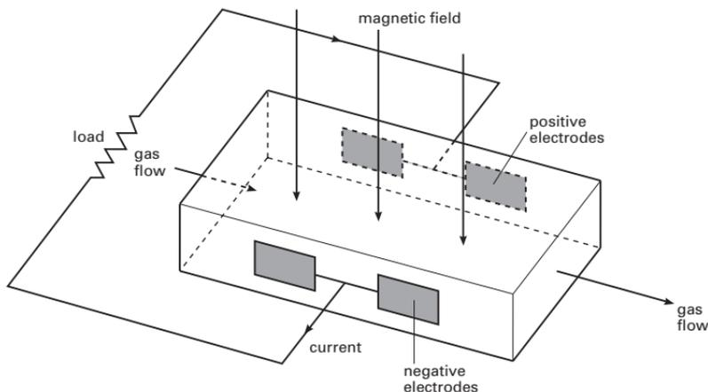
**Magnetohydrodynamics.** Magnetohydrodynamic generator.
