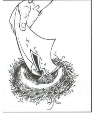
"Sparking" mish-metal insert to ignite shavings by pulling up on magnesium bar.
