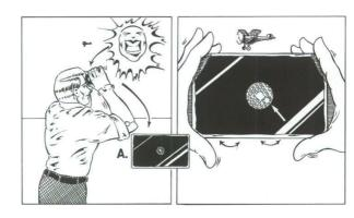
Locate target within sighting hole while keeping track of glowing ball of light.
