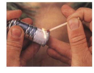
The magnesium block with striking insert. The yellow tape and yellow hacksaw blade help with visibility.
