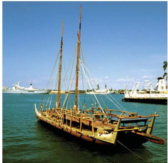
The Hokule'a is a reconstruction of the type of canoe the ancient Polynesians would have sailed on long sea voyages. The Polynesian Voyaging Society of Hawaii has successfully sailed the Hokule'a and other such canoes throughout the Pacific without using modern navigational instruments.
