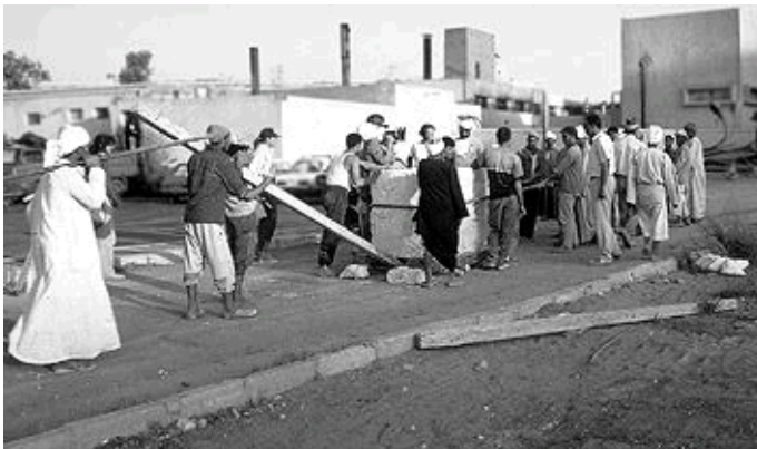
Figure 72: NOVA pulling of stone on rollers was only feasible on a flat hard surface, like modern road. It did not work on sand.
