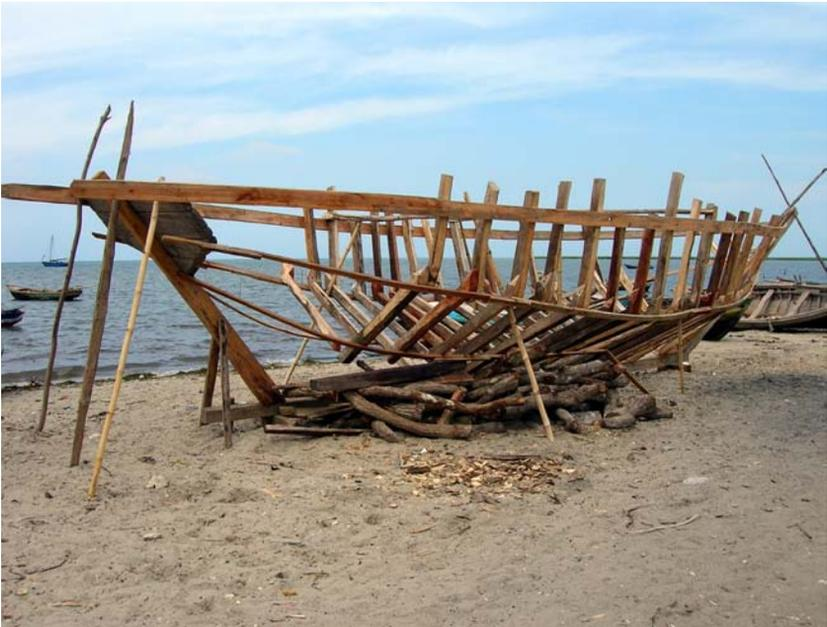
*Fig. 3.1.* A traditional wooden 'skeleton-first' fishing boat being built on the beach at Petite-Anse in Cap-Haitien, Haiti. As can be clearly seen, the frame or 'skeleton' of the vessel is erected first. Once in position, the planking of the hull is then nailed directly to the ribs of the vessel. Photo: Rémi Kaupp.
