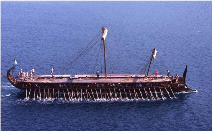
*Fig. 3.9.* The replicated trireme *Olympias* under oars during sea-trials off Poros in 1988. Photo: Courtesy of The Trireme Trust.
