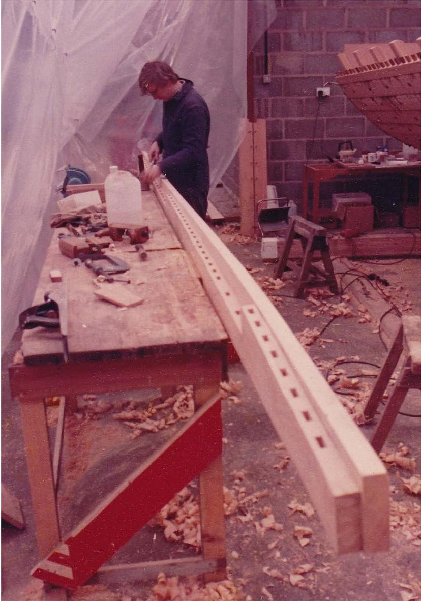
*Fig. 3.2.* The ancient shell-first method of ship construction. A shipwright cutting mortice holes into a garboard on a trial section of a replicated Classical trireme. Picture courtesy of Malcolm Adkins.
