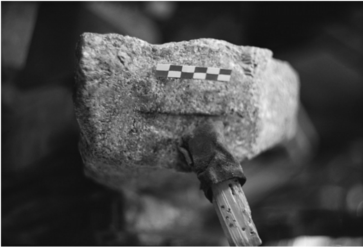
Figure 3.16 Polishing the granite with a leather lap and mud
