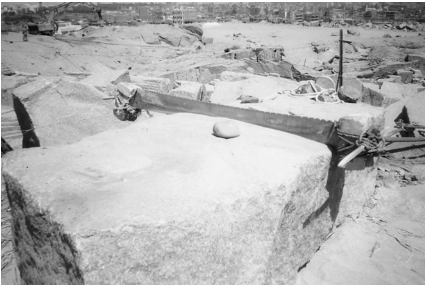
Figure 6.3 A stonecutting saw needed to be slightly longer than the width of a block of stone, to allow for its reciprocating movement
