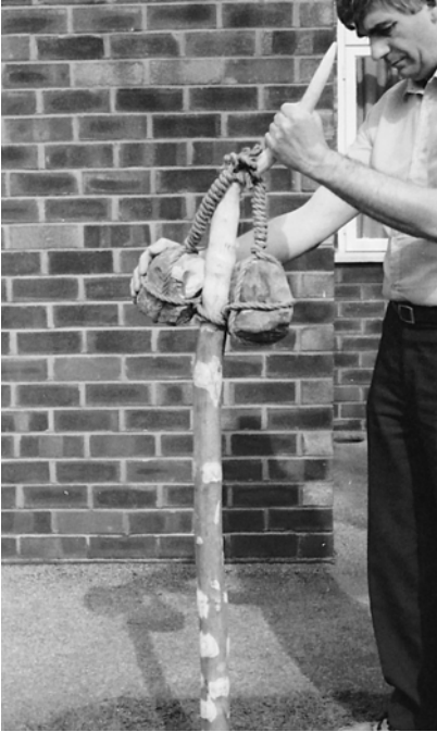
Figure 5.21 A clockwise twist of a large drill-shaft
