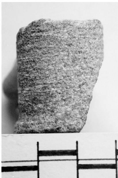
Figure 4.17 Striations cut into a stone core
