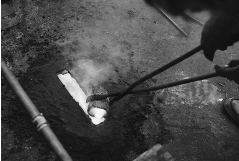
Figure 2.15 Casting a flat-edged copper saw blade in an open sand mould
