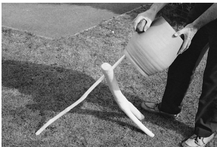
Figure 2.32 Demonstrating the tripod anvil, adjusted for use with a large vessel
