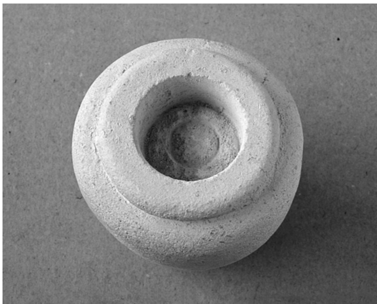
Figure 5.32 The tubular core is now removed
