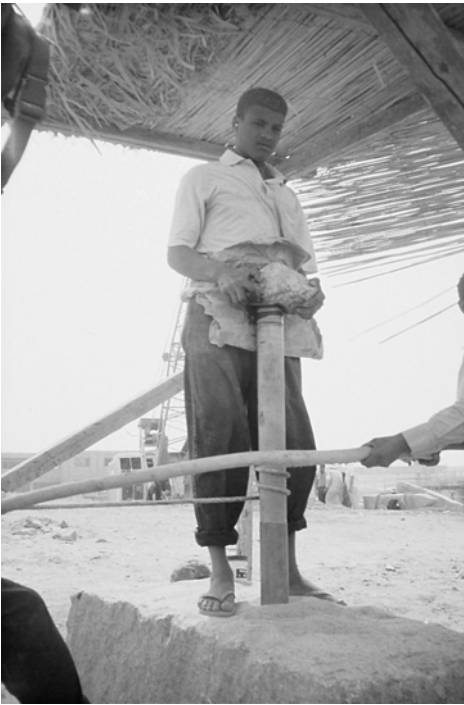
Figure 4.22 The bow-rope double turned around the drill-shaft
