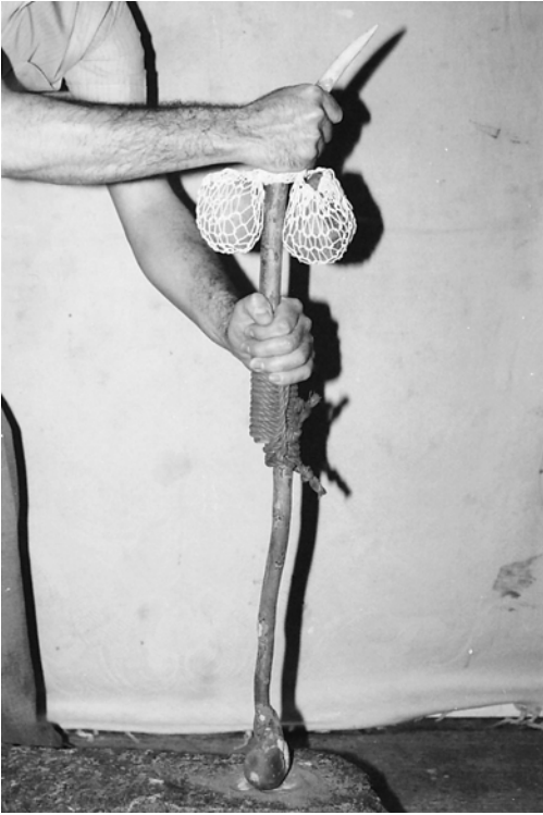
Figure 5.19 A TRTD, fitted with a forked shaft, driving a stone borer
