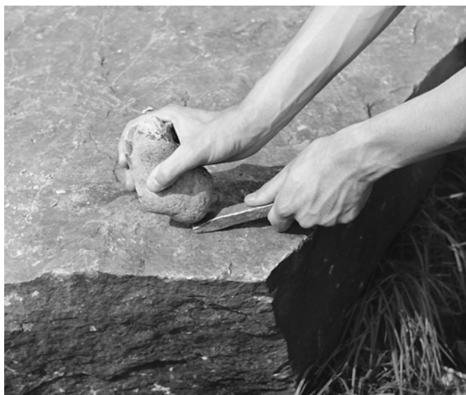
Figure 2.50 Hammering a bronze casting into a chisel
