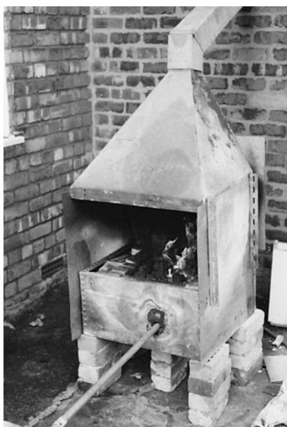
Figure 2.48 The author's furnace for melting copper and bronze
