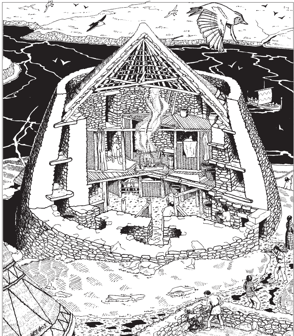
A cutaway drawing showing life in the broch tower of Dun Carloway, Lewis. The ground floor is used for animal shelter and storage, while domestic activity is concentrated on the upper floors.
