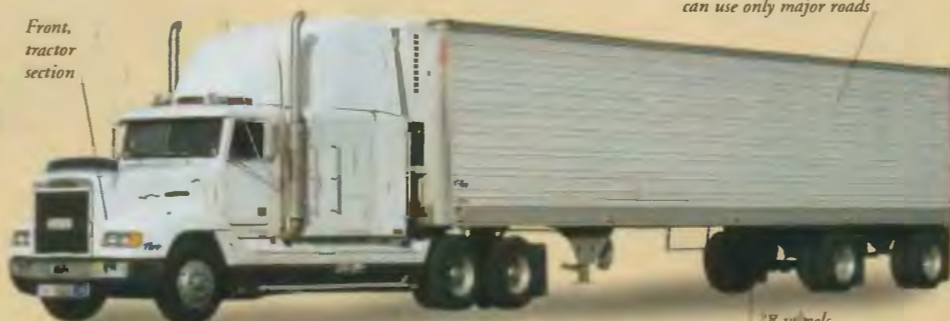
Semitrailer: a monster truck suitable for a wide range of bulk or heavy goods
