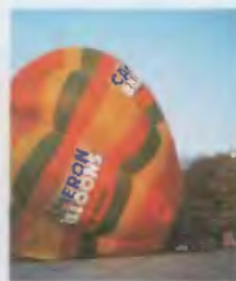
2 The balloon's envelope expands as the hot air starts to fill it
