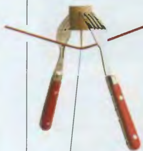
Centre of gravity is directly below the string, making the object very stable.
