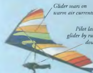
Hang glider is like a huge wing with a harness below to hold the pilot.
