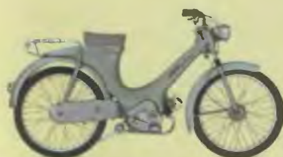
Heinkel Perle, 1956, has all the wires and cables running from the handlebars through the frame.
