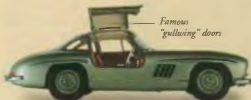
Mercedes-Benz 300SL, Germany; launched 1954; top speed 265 kmh (165 mph)
