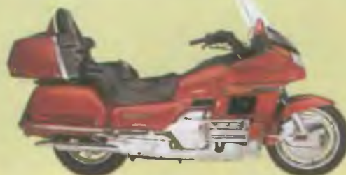
Honda GL1500/6 Gold Wing, 1991, has a 1500cc engine, an extra pair of cylinders, and luxuries such as a cassette player.
