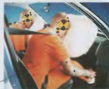
Testing airbag inflation
