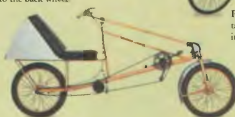
Triple tandems have three sets of pedals for three riders, linked by a chain to the back wheel.
