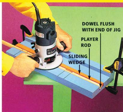
Photo 3 • Clamp down the routing jig and wedge each dowel firmly in place, flush at the right end. Keep the router base against the rear fence when cutting grooves.
