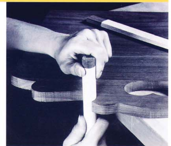
Photo 3 • Sand the curved edges with sandpaper taped to a dowel, or use a sanding drum mounted in an electric drill or a drill press.
