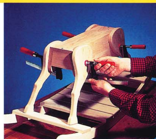
Photo 5 • Clamp the legs to the body and set the horse on the rocker. Adjust the leg positions, then turn the assembly over to screw the legs to the body from the inside.
