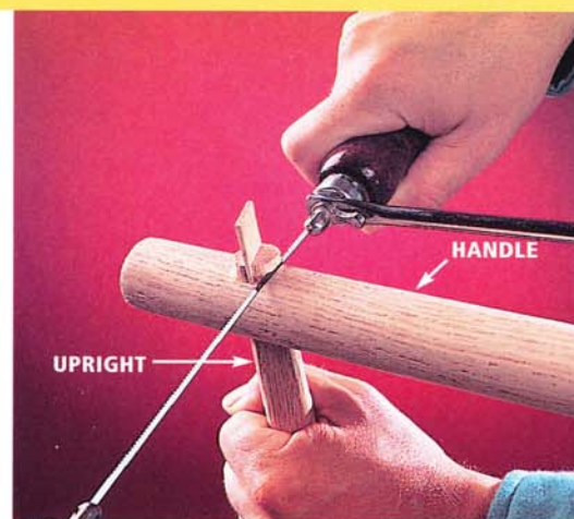
Photo 3 • Use glue and wedges to secure the uprights in the handle. Cut off their ends and sand them flush with the curve of the handle.
