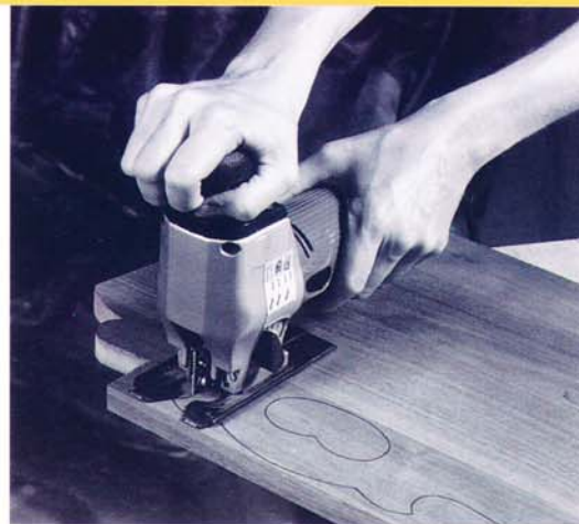
Photo 2 • Transfer and enlarge the patterns onto the wood, then cut the scrollwork with a saber saw or jigsaw.
