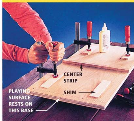
Photo 1 • Glue the shims and center strip to a plywood base so the playing surface will bend over them and gently slope toward each end.
