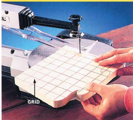
Photo 1 • Cut out one of each curved part and sand the edges. Trace the duplicate parts from the first, for an exact match.
