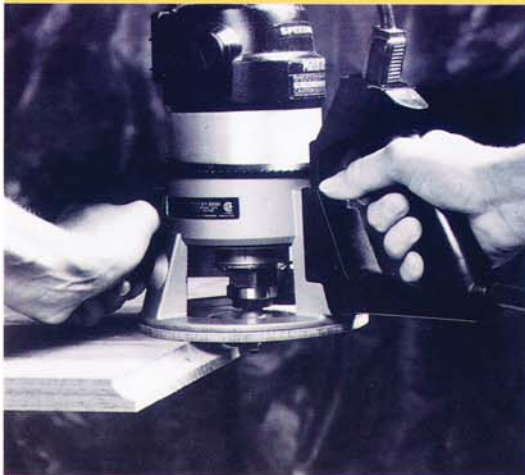
Photo 1 • Rout the edges of the cradle bottom with a 1/2-inch self-piloted cove bit, making several light cuts.
