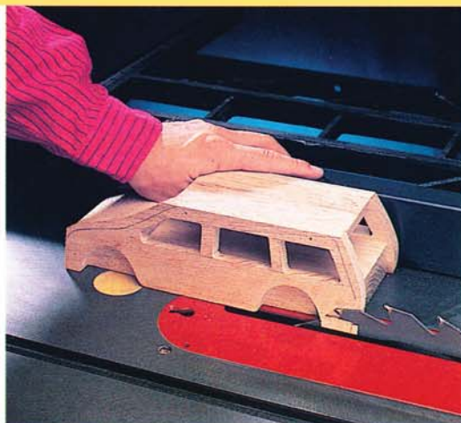
Photo 2 • Rip the sides to make a vertical face on the lower half. This gives the minivan a distinctive, more realistic look.
