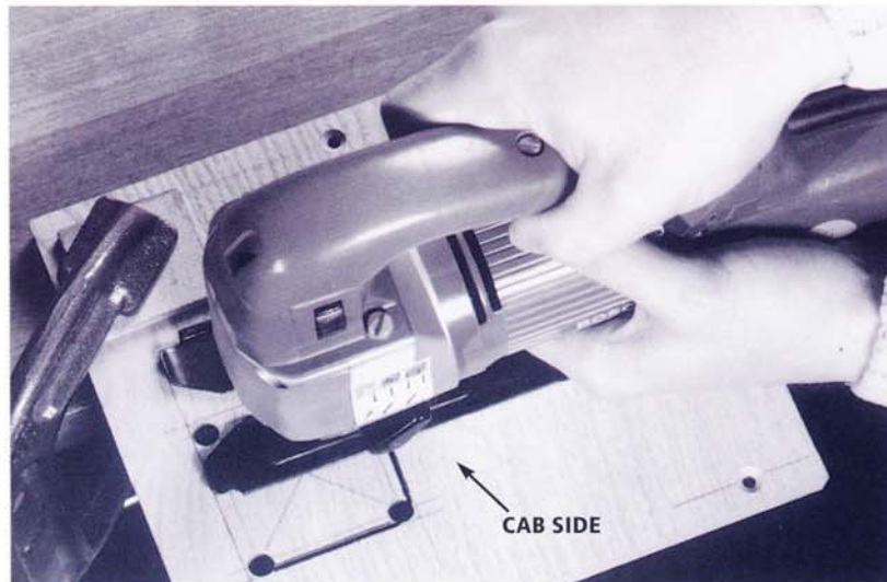
Photo 3 • To cut out the cab windows, drill 3/8-inch holes at each corner, then cut between the holes with a saber saw.
