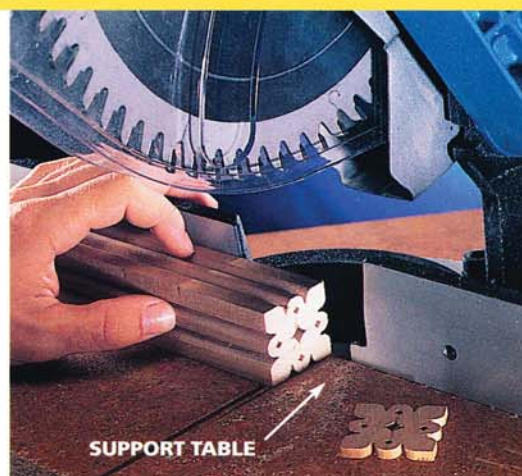
Photo 3 • Rout the glued-together stick, then crosscut it into slices. Use an auxiliary table to support the slices.
