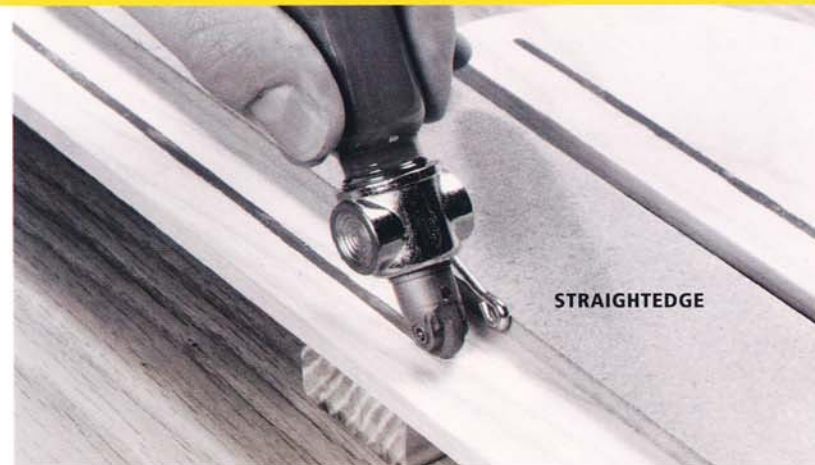
Photo 9 • Clamp a straightedge in place to guide the pinstriping tool. Practice the striping technique on scrap wood until you feel comfortable with it.
