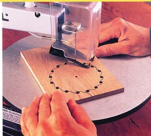
Photo 2 • Drill a series of 1/4-inch holes to make uniform gullets in the blade. They also make the piece easy to turn when cutting it out.
