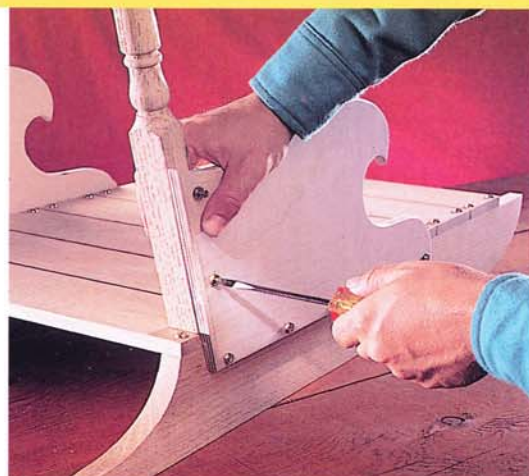
Photo 2 • Test-assemble the sled with steel screws. Disassemble it to apply the paint and varnish to the parts and reassemble with brass screws.
