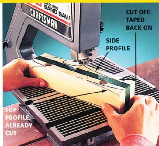
Photo 2 • Cut the top body profile first, then tape or hot-melt glue the cutoff pieces back in place to cut the side profile. Pry glued pieces apart with a putty knife or other thin blade.
