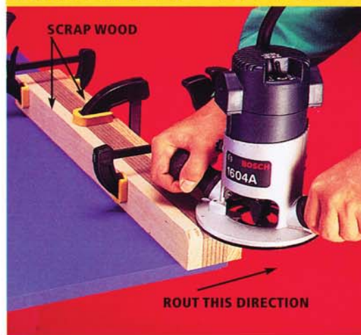
Photo 3 • Gang the hardboard frame pieces between two pieces of scrap for routing, to make all pieces exactly the same shape. Use a 1/2-in. diameter round-over bit.
