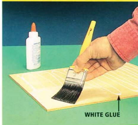
Photo 2 • Spread a thin, even coat of white glue over the face of the plywood with a fine-bristle paintbrush.
