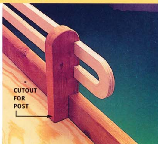
Photo 9 • Notch the plywood bed bottom to accommodate the guardrail posts and help hold them in place.
