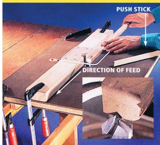
Photo 1 • Use a router table to cut V-grooves 3/32 inch deep on two sides of 3/4-inch square sticks. Other grooves are cut after gluing-up.
