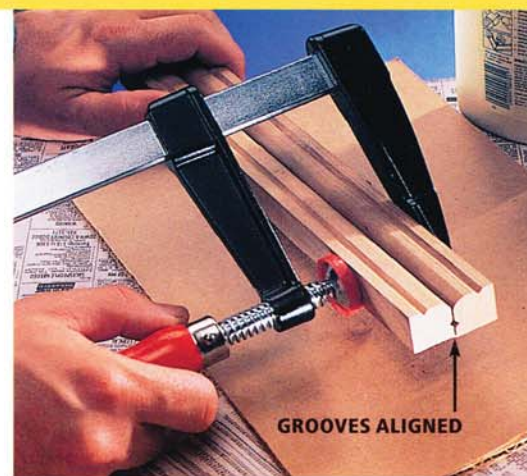
Photo 2 • Glue pairs of sticks together. Align the V-grooves exactly and be careful to avoid glue squeeze-out; it will be hard to clean up.
