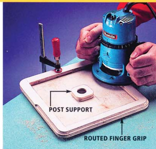
Photo 2 • Rout finger grips on the bottom edges of both bases. They make it easy to separate the bases when they are held by the Velcro closures.
