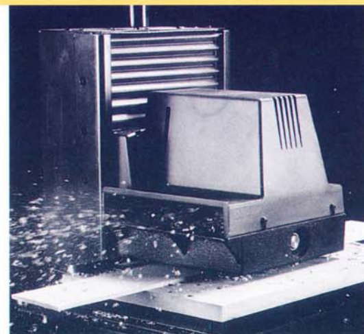
Photo 2 • Plane boards to finished thickness, taking material off both sides. This relieves internal board stress and prevents cupping.
