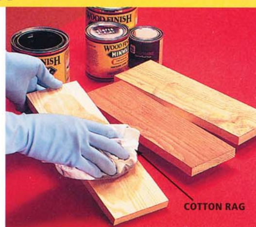
Photo 6 • Make tests on scraps of pine to find how to stain to the depth of color you want. Use oil-base stain, with a stain controller to avoid blotching if necessary.
