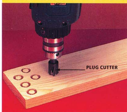
Photo 5 • Cut plugs to cover the screws using a 3/8-inch plug-cutting bit. To keep the bit from wandering, position it against the wood, then start drilling.
