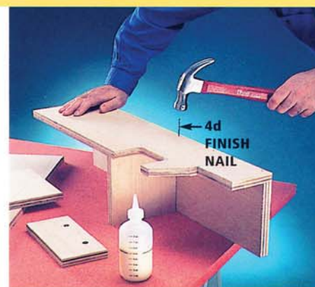
Photo 3 • Glue and nail the body parts together. Locate the 4d finish nails in the top at least 3/8 inch back from the edges so they won't interfere with rounding over the edges later.
