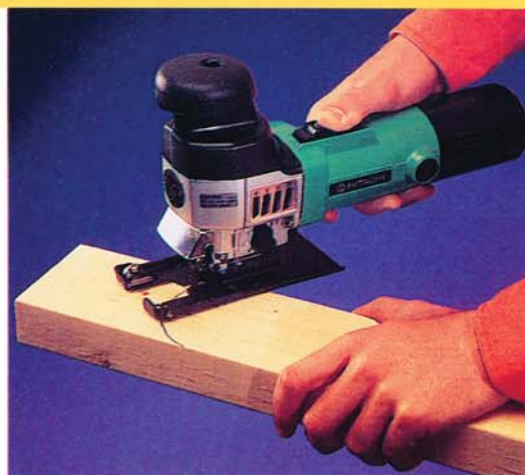
Photo 2 • Cut rounded ends with a saber saw and a fine-tooth blade. Smooth the cut faces with a file or belt sander.
