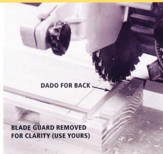
Photo 4 • Cut the long 1/2-inch dados in one pass. Cut each short, wide dado in several passes, until the width matches the thickness of the back.
