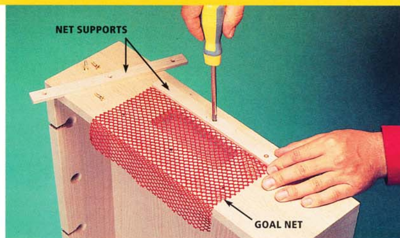
Photo 7 • Align the nets and net supports over the goals. Drill pilot holes and insert the screws through the supports and net mesh before driving them into the holes.
