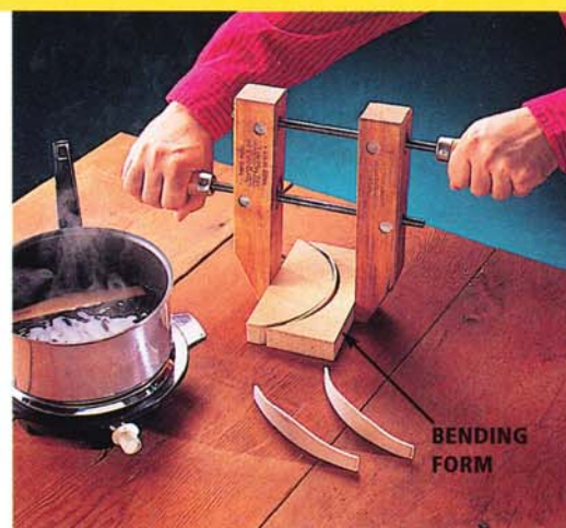
Photo 3 • Bend the slats by boiling them for half an hour and then clamping them overnight in two-part bending forms.
