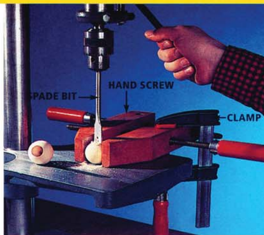
Photo 7 • Drill holes partway into the birch balls that finish the ends of the handle. Use a hand screw to hold them; clamp the hand screw to your drill press bed or work surface.
