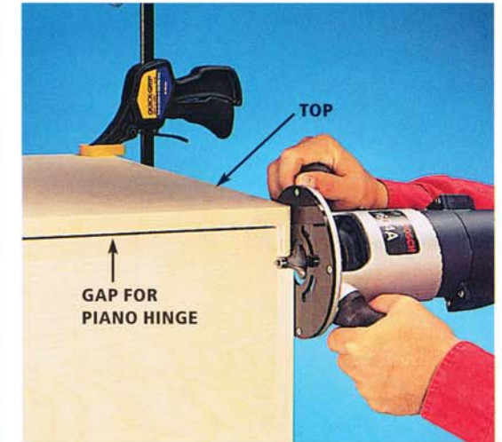
Photo 2 • Round the corners of the top this way. It will prevent accidentally rounding over the bottom edges of the top or tearing out the wood.
