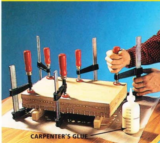
Photo 1 • Glue and clamp the three head blanks together. Make sure the edges remain aligned while you install the clamps.
