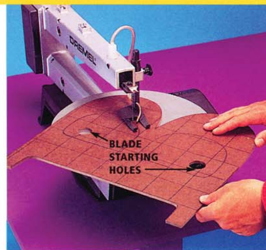
Photo 4 • Cut the outside shapes of the letters with a jigsaw. Then drill starting holes in the letters "A" and "B" to insert the blade for cutting out the inside shapes.
