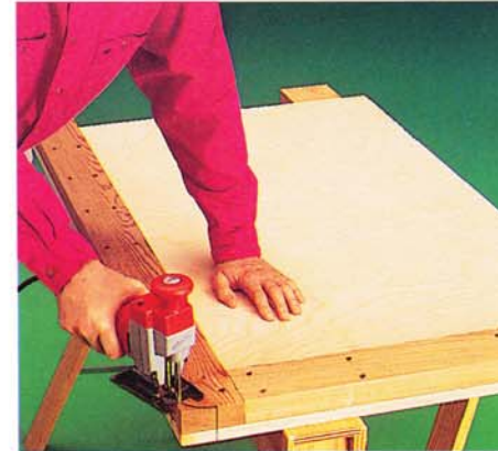
Photo 7 • Cut rounded corners on the desktop after screwing 2x4's under the front and left sides. Set the 2x4's flat and flush with the edges of the plywood.
