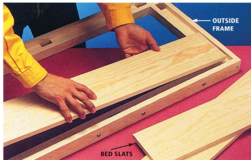
Photo 1 • Build the frame assembly for the wagon bed. Then position the bed slats, drill pilot holes, and screw the slats to the frame assembly.
