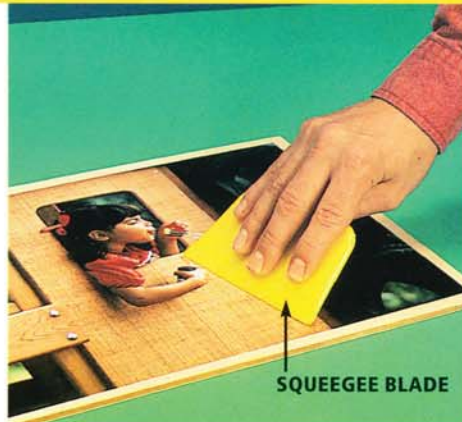
Photo 3 • Press the picture into the glue with a squeegee. Use light pressure to work out air bubbles under the paper.
