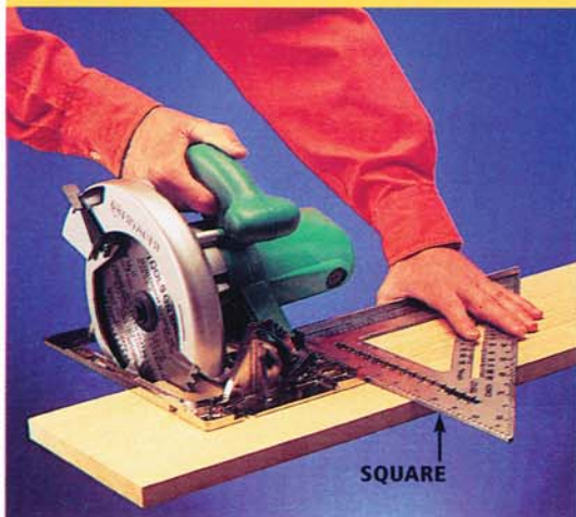
Photo 1 • Use a square as a saw guide to crosscut square ends on boards. Use a straight board as a guide for longer cuts.
