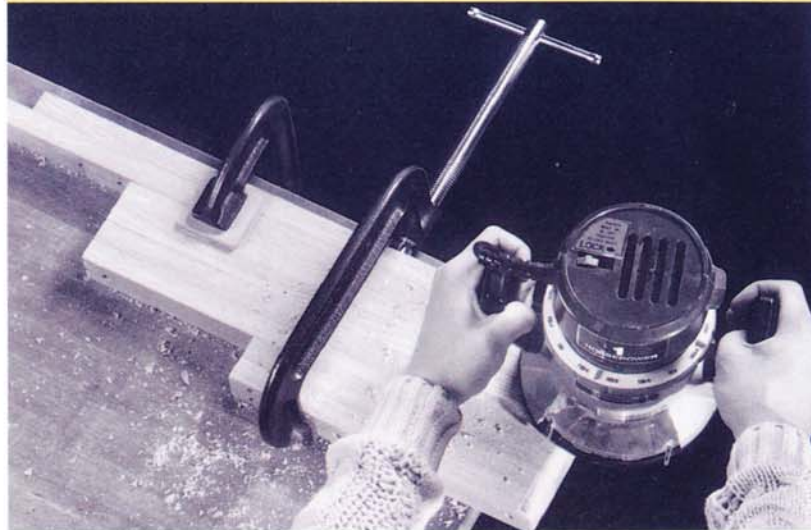
Photo 2 • Round over the ends of all the shovel arms at once. Clamp them together and to a bench and rout them in one pass.
