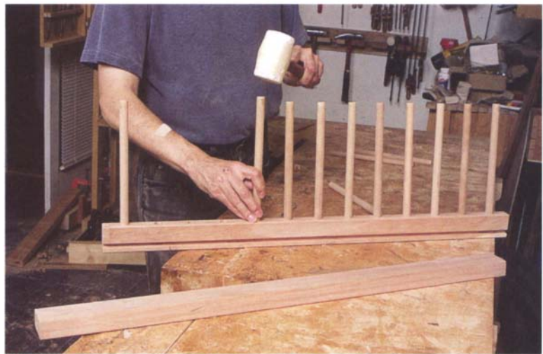
PHOTO E: Insert all of the dowels into one of the lower side rails first.
