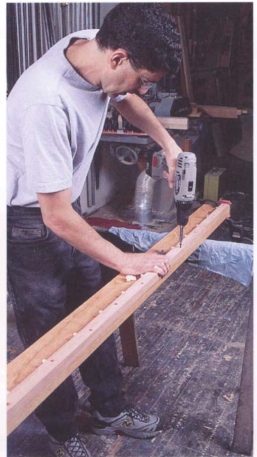
PHOTO I: Start at one end of the cleat, clamp it into place, and tighten down the first screw. Then work your way across, making sure the cleat remains flush with the bottom of the rail as you go.
