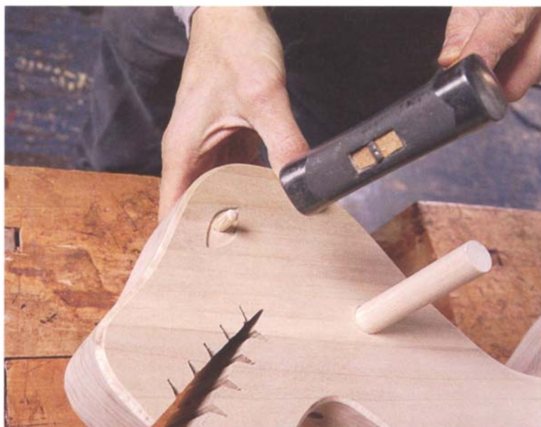
PHOTO C: To make the pupils, tap ¼-in. dowels, which have the ends rounded over, into the holes in the eyes. Tap until only the rounded part of the dowel is exposed.
