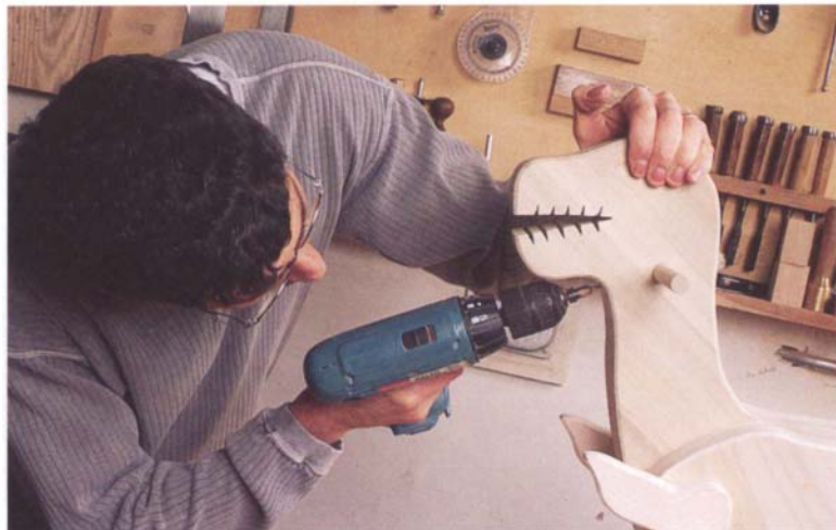
PHOTO J: Aim your drill toward the handle; then drill and screw to lock the handle in place.
