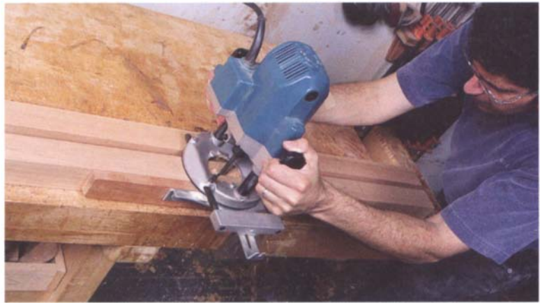
PHOTO D: Clamp the post to the bench before routing the head-board mortise. Use a second leg, also clamped to the bench, to help support the router during the cuts.
