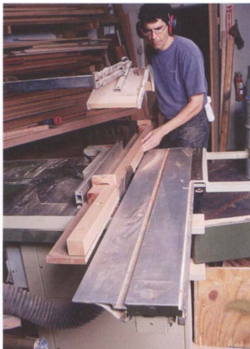
PHOTO F: When tapering the posts on a table saw, you'll need an outfeed roller or an assistant to support the long posts with jig as they leave the saw.
