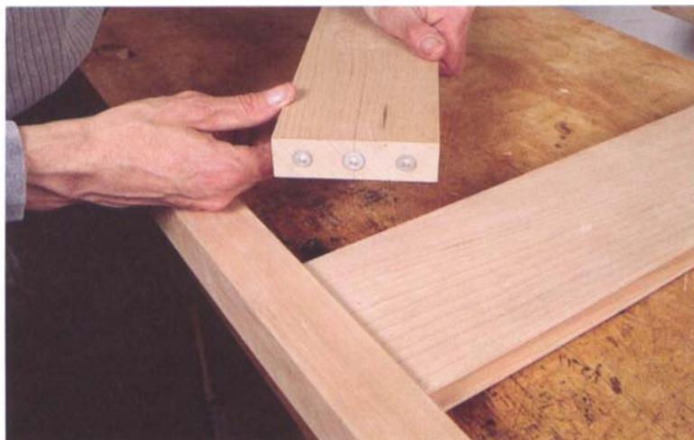
PHOTO E: Dowel points transfer the exact locations of the holes in the end of the inner front rail to the inside of the lower end rail.
