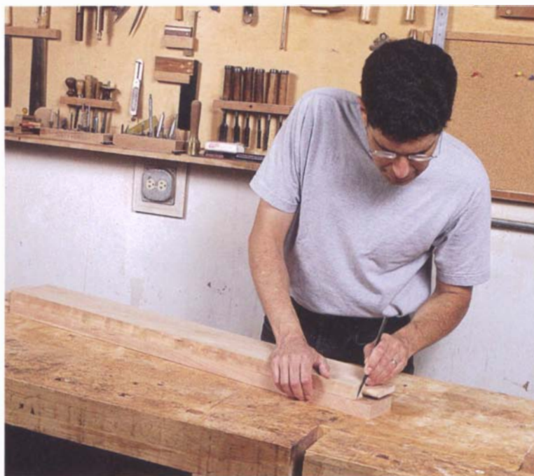
PHOTO A: Use the lower rail as your ruler for marking out the length of the upper rail between the shoulders. With the shoulders on one end perfectly flush, scribe the location of the opposite end of the upper rail from the lower rail shoulder.
