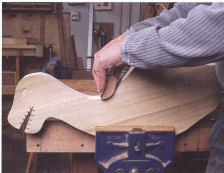
PHOTO B: Tighter curves can be sanded with a sanding block that roughly matches the curve to be smoothed.
