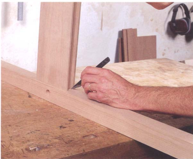
PHOTO C: Transfer the location of the panel groove from the rail onto the leg by marking with a knife.
