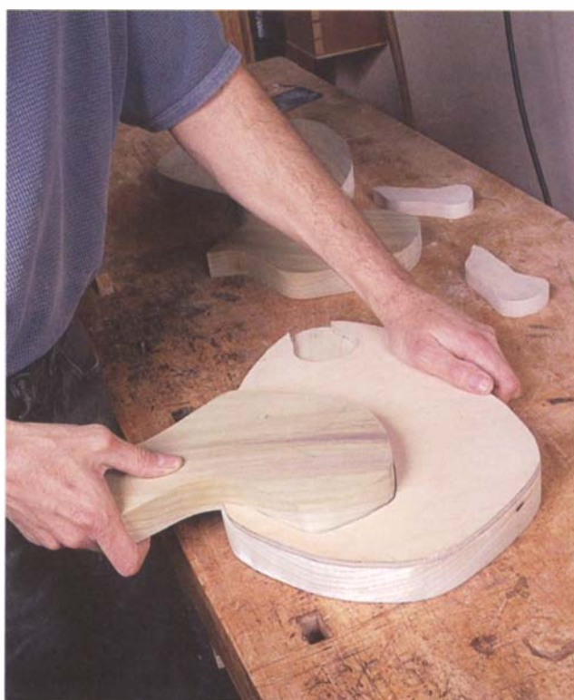
PHOTO D: With the shape of the leg cut out of it, the flank pattern helps locate the legs in the same place on both sides of the dinosaur.
