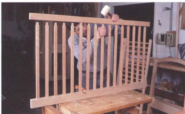
PHOTO H: Starting at one side and working across makes assembly a one-person job. I use a non-marring rubber mallet to tap each slat into its mortise.
