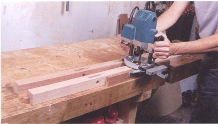
PHOTO D: Using the second leg as a support for the router makes routing the groove for the panel safer and more accurate.
