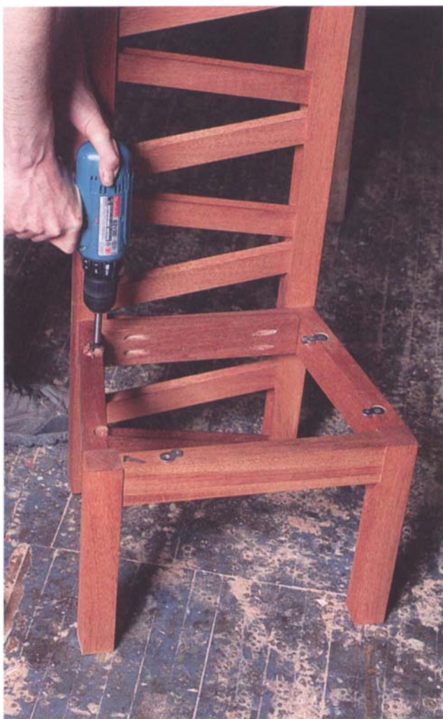
PHOTO J: The shallow holes for the figure-8 fasteners have to overlap the inside edge of the rail. Use the fastener itself as a guide in determining how much overlap you need.
