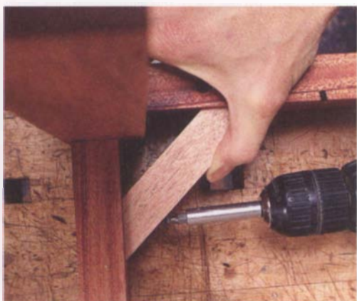
PHOTO E: There's enough room inside the aprons to use a cordless drill to drive the screws into the corner blocks.
