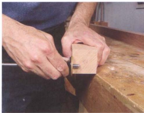
PHOTO E: Marking the top of the posts for tapering is quick and accurate if you use a marking gauge.
