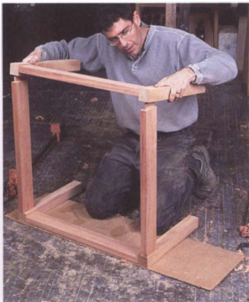
PHOTO D: Fit the aprons to one sub-assembly, carefully work the opposite subassembly into place, and then add clamps.
