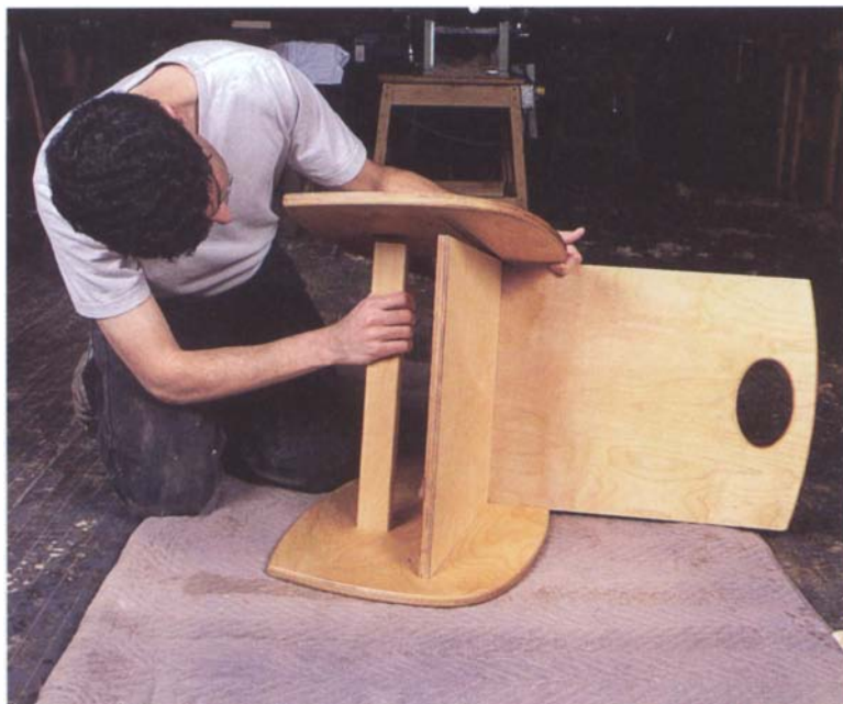
PHOTOS G AND H: Assembling the rocker can be frustrating without help. It makes sense to do it on a blanket or a piece of cardboard in case something slips apart.
