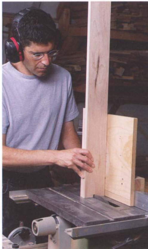
PHOTO J: The slots in the ends of the slats can be cut easily on the table saw, using a tenoning jig with a wooden fence attached to support the slat.
