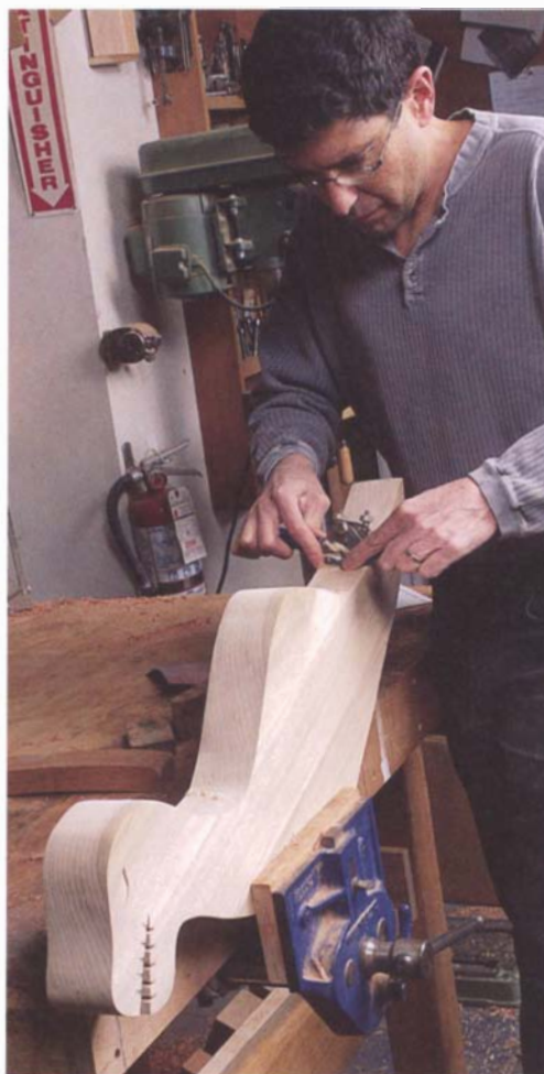
PHOTO A: A spokeshave works well for smoothing both the convex and the shallower concave sections of the body parts.
