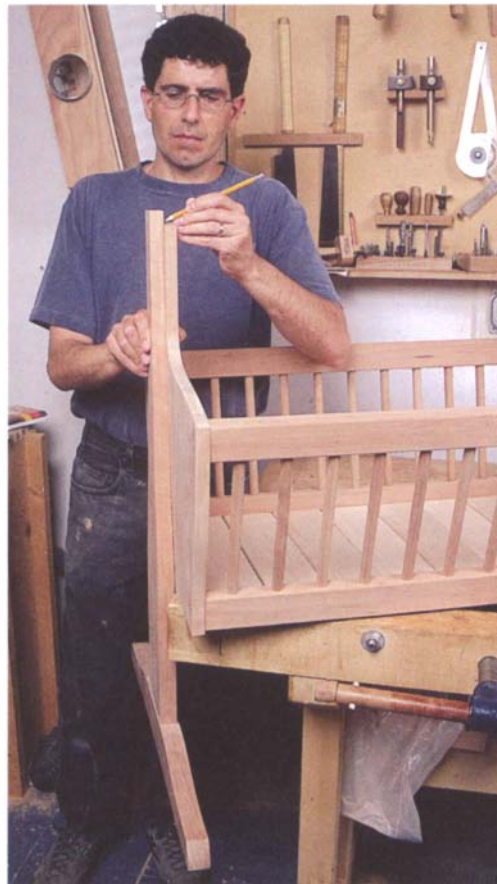
PHOTO H: Scribe the top of the base uprights directly from the basket ends so they match perfectly.
