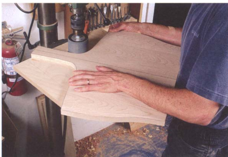
PHOTO B: The part of the basket end that's hard to sand by hand is easy to sand with a sanding drum mounted in the drill press.
