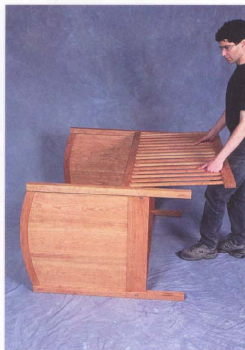
PHOTO J: Slide the front drop gate up the groove in the front legs.
