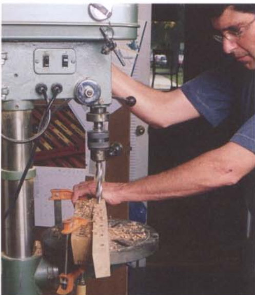
PHOTO C: Clamp the angled drilling fence to the drill-press table to drill the \frac{5}{8} -in. holes centered on the rails.
