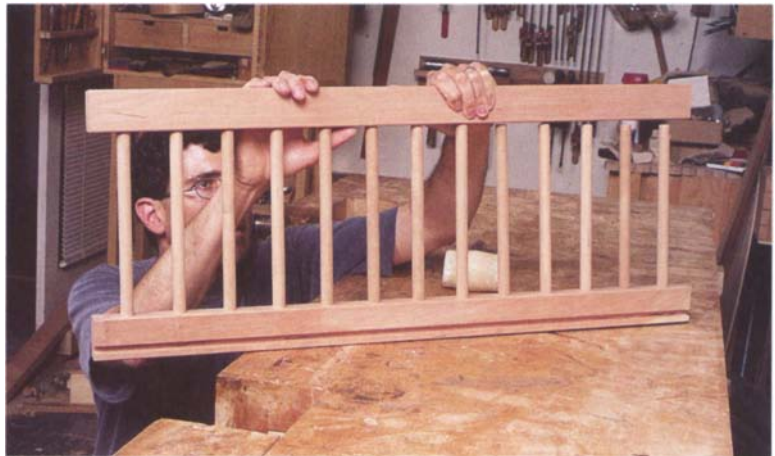
PHOTO F: The upper rail goes on to the lower rail and dowels one dowel at a time, starting at one end. Once the dowels are all in place, clamp the rails to be sure the dowels seat all the way.
