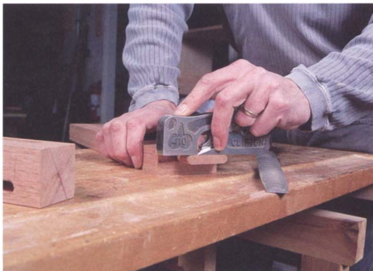
PHOTO G: The rabbeting plane is designed for fitting tenons. You can also use a rasp or sandpaper on a block. Whatever your tool, be careful not to taper or round over the face of the tenon.
