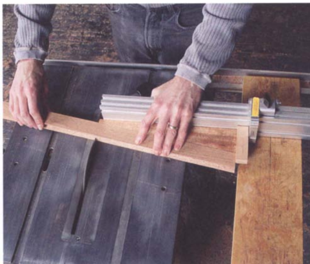
PHOTO C: The chair wedge ensures that all of your rung cuts are the same, but it also will do much more throughout the project.
