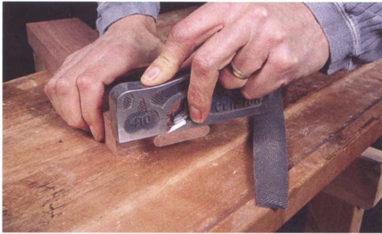
PHOTO B: Fitting tenons is what a rabbet plane does best. Hold the plane flat and cut across the grain.
