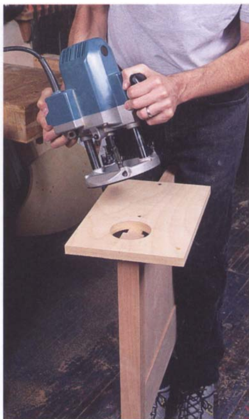
PHOTO G: The leg-trimming jig makes it easy to rout the top of the leg perfectly flush with the upper rail.
