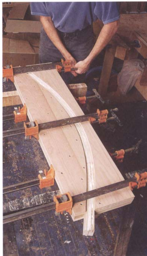
PHOTO F: The clamps should alternate between top and bottom to provide even pressure. You'll need at least five or six heavy-duty clamps.
