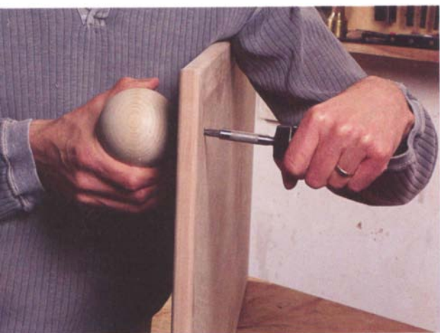
PHOTO F: Hold the ball foot to keep it from turning when you tighten the screw.
