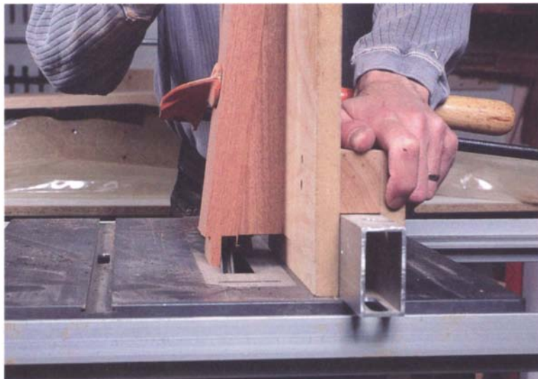
PHOTO F: An angled tenon is no more difficult to cut than a straight one, once you have the wedge attached to the tenoning jig. Note that the tenon is angled but the shoulders are perpendicular to the tenon.
