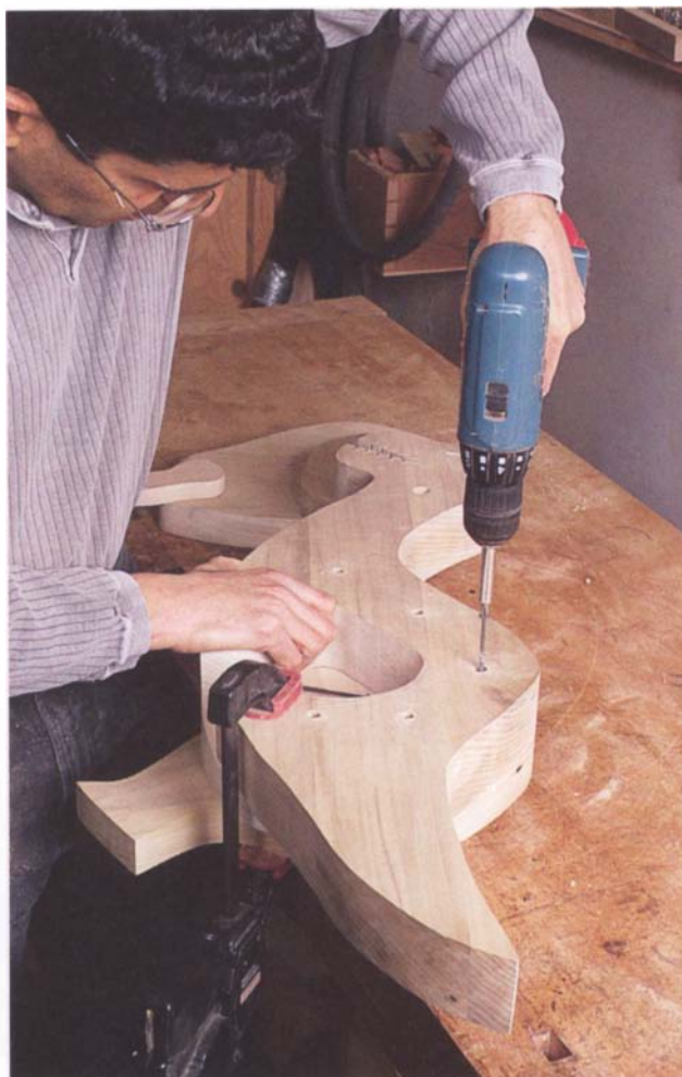
PHOTO E: Screw one flank to the main body from inside. The second flank has to be screwed on from the outside.
