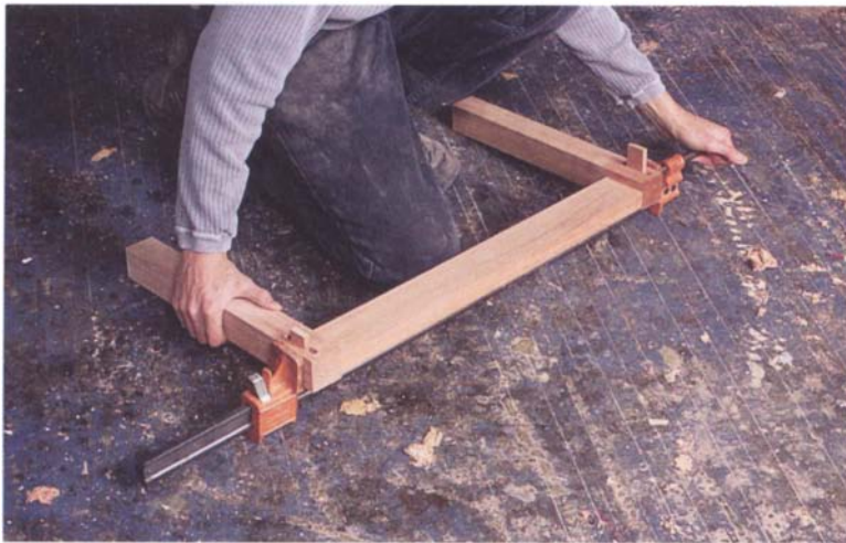
PHOTO C: Gluing up in two stages is a much calmer process than doing it all at once. Start with gluing the legs to two (opposite!) aprons. Filler blocks keep the apron mortises from being crushed.
