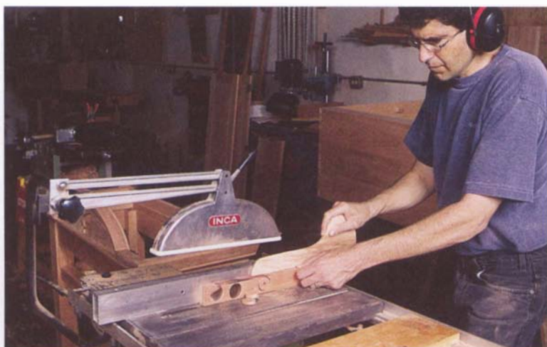
PHOTO I: Cutting the drilled spacers out of the block is a straightforward process on the table saw.
