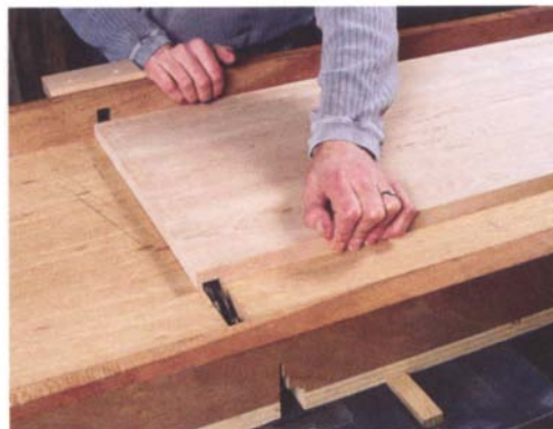
PHOTO A: Cut the dados on the front and rear panels on the table saw. A crosscut sled makes the job safer and easier.
