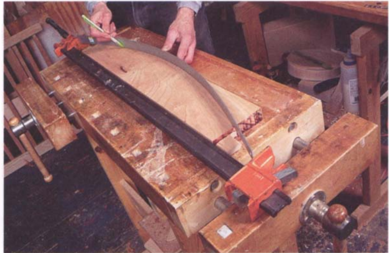
PHOTO C: Springing a 3-ft. ruler or a thin strip of wood with a clamp is an easy way to lay out a curve. Adjust the curve by tightening or loosening the clamp until you have the curve you want.
