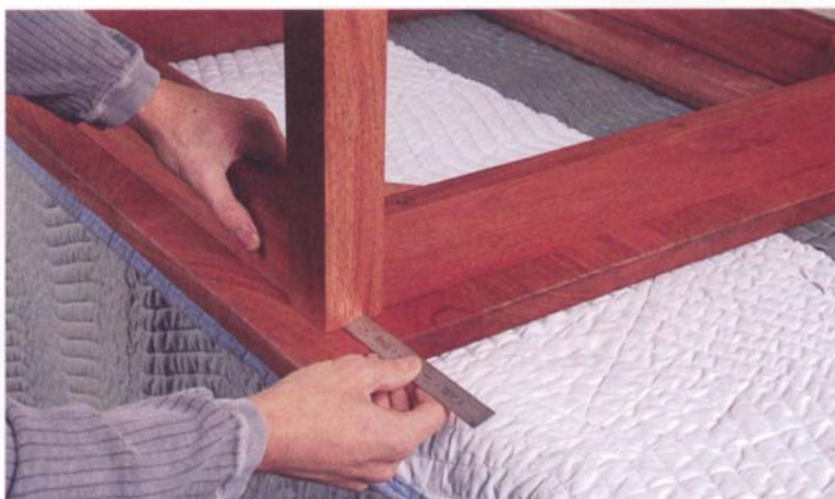
PHOTO H: Take time to get the base centered on the top. Measure from both faces of all four legs. When the base is properly positioned, hold it tightly in place and drive in the screws.
