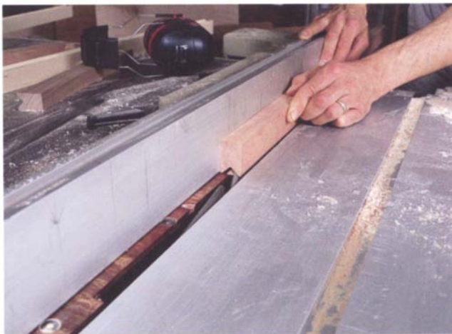
PHOTO B: Use the same fence setting for both of the cuts to make the V-groove. Turn the rung stock around for the second cut. It's important for safe handling on the saw to retain the narrow flats on either side of the V-groove.
