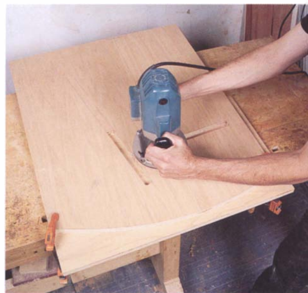
PHOTO B: The dados in the side panels are easy to rout, and they come out in exactly the right place if you use the dado jig.
