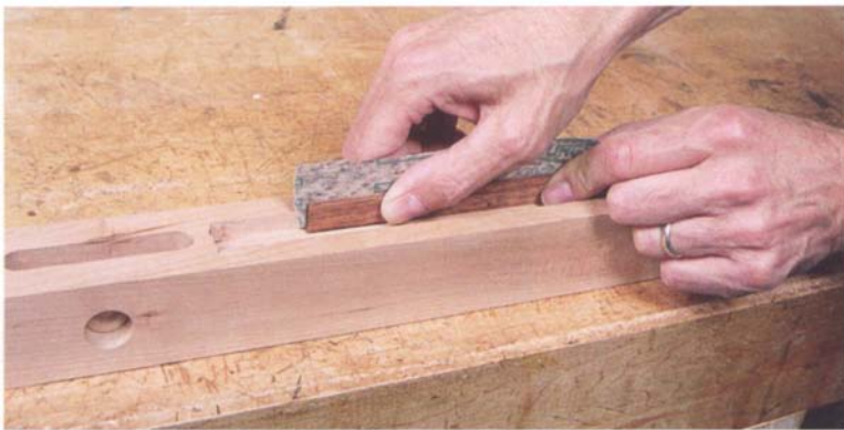
PHOTO E: The grooves in the legs and the rails must line up exactly. Selective sanding of the sides of the panel groove in the leg can help correct a minor misalignment.
