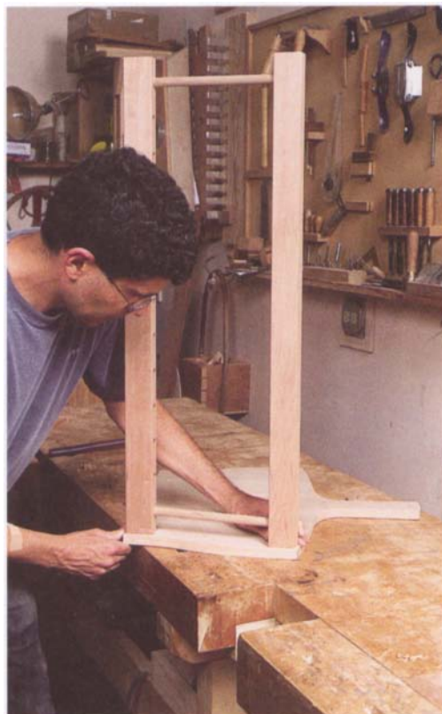
PHOTO D: The actual length of the dowels should be determined by checking the result of a test-assembly against the basket ends.
