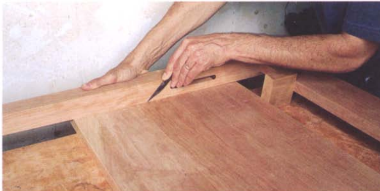
PHOTO I: To scribe the shoulders of the headboard, place the headboard blank over the headboard post-and-rail assembly. Note the spacer blocks, which help position the headboard the proper distance from the top edge of headboard rail.
