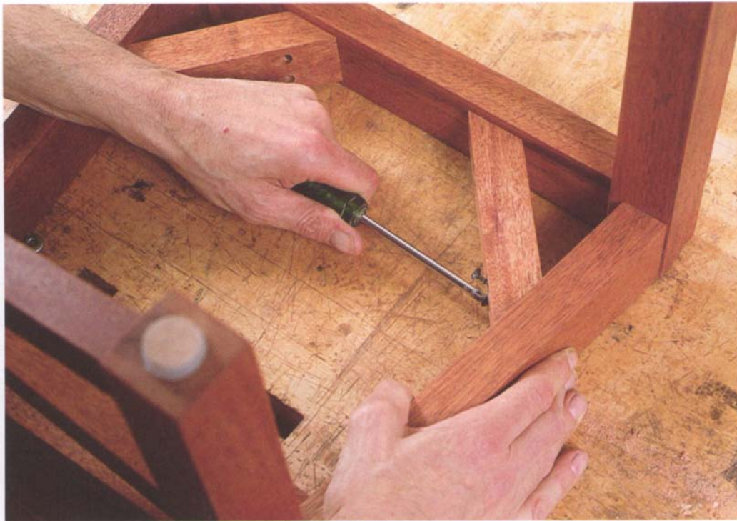
PHOTO K: Hold the corner block in place and screw into the front rail and then the side rail.
