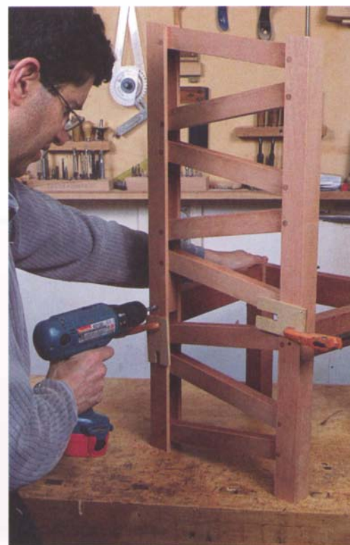
PHOTO H: The connector-bolt hole in the back leg guides the drill into the back of the side rail.
