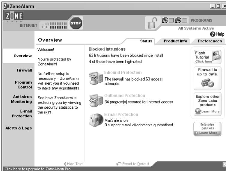
**Figure 10-12** The ZoneAlarm firewall's main console displays how many possible intrusions it has blocked and how many programs are secured for Internet access.
