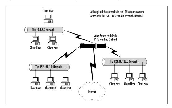
Figure 9.1 A Linux System Configured as a Forwarding Router
