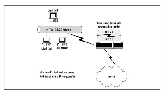
Figure 9.2 Masquerading the 10.1.2.0 Network as the 66.1.5.1 IP Address
