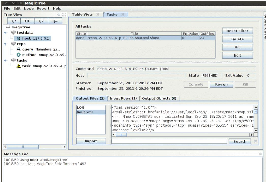
We will select `$out.xml` and click on the **Import** button to have MagicTree automatically generate our node structure based on the scan results.
