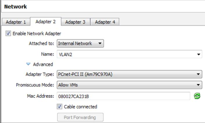
The screenshot shows the configuration for Network Adapter 2 in pfSense. The 'Network' section is active, and 'Adapter 2' is selected. The 'Enable Network Adapter' checkbox is checked. The adapter is attached to the 'Internal Network'. The name is 'VLAN2'. Under the 'Advanced' section, the 'Adapter Type' is 'PCnet-PCI II (Am79C970A)', 'Promiscuous Mode' is 'Allow VMs', and the 'Mac Address' is '080027CA231B'. The 'Cable connected' checkbox is checked, and there is a 'Port Forwarding' button.
