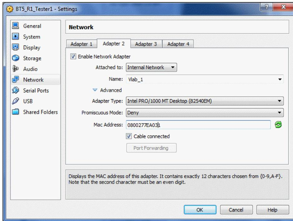
16. Click on the **Adapter 2** and select the **Enable Network Adapter** checkbox.
