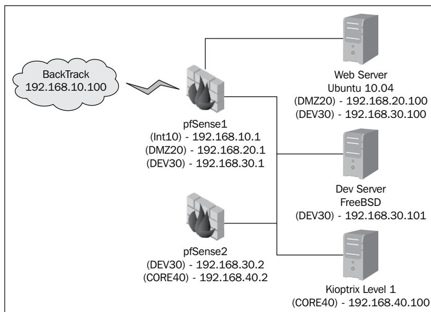
In this whitebox test we were provided with the network architecture to make up for the fact that we are testing a mock environment and are limited by a strict timeframe. We need to determine if the router will let us through from pfSense1 to the WebServer and to the DevServer. It is unclear from the provided diagram if we can reach the Kioptrix Level 1 machine remotely or not. Our initial plan is as follows:
