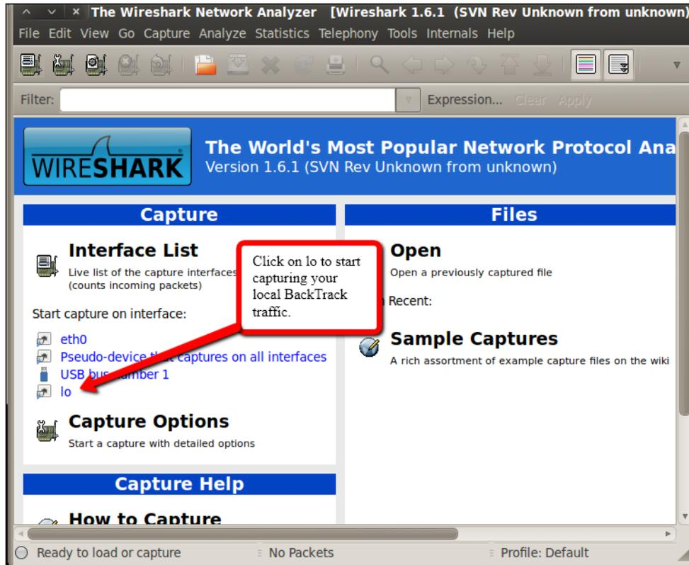
Let's reproduce the error, but this time we will watch the packets in **Wireshark** as they traverse the local loopback interface. Restart the `vulnserver`, and then start `bed.pl` again using the `vserver` plugin. Once everything has started click over to Wireshark and take a look at the packets that are being passed. You can right-click on any of the messages in Wireshark and select **Follow TCP Stream** to see the messages in an easy to read format.
